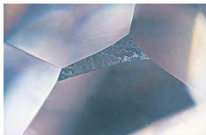
Figure 10. Magnification at 30× reveals etching on one of the pavilion facets of the 7.54 ct diamond. This feature suggests that the diamond was subjected to the extremely high temperatures used in HPHT processing.
