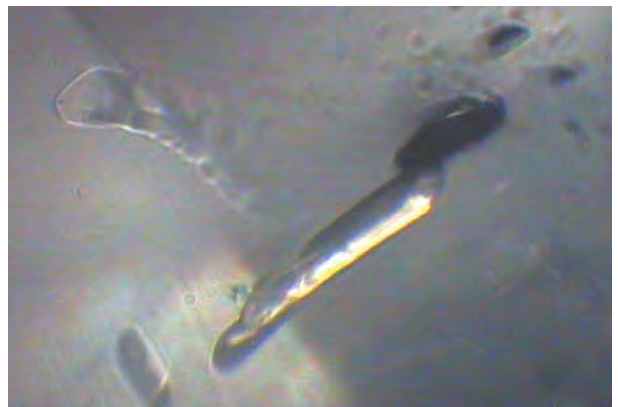
Figure 10. This colorless elongated zircon inclusion measures 0.20 mm long. Photomicrograph by A. Donini.
