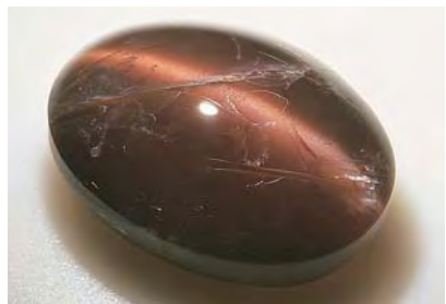
Figure 11. The inclusions (possibly hematite) that cause the chatoyancy in this 25.98 ct “blood-shot” iolite are also responsible for the orange color of the eye.
