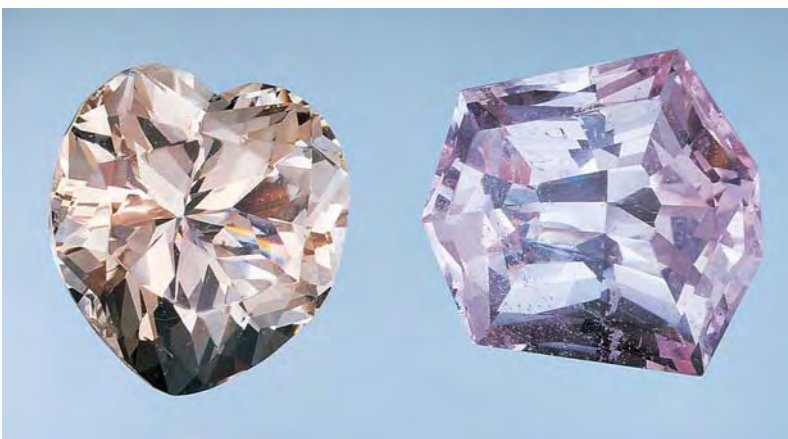
Figure 7. The 191.59 ct stone on the left shows the brownish pink color that is typical of morganite as it is mined from the White Queen mine in Pala, California. After exposure to sunlight for about one week, the brown color disappears, as shown in the 202.41 ct purplish pink White Queen morganite on the right. Courtesy of Bob Dawson; photo © Harold & Erica Van Pelt.
