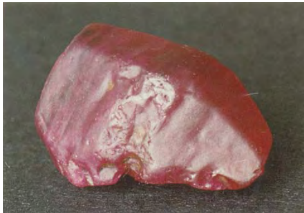
Figure 38. This 9.56 ct broken bipyramidal "crystal" was actually manufactured from low-quality flame-fusion synthetic ruby. Photo by Jaroslav Hyrsl.
