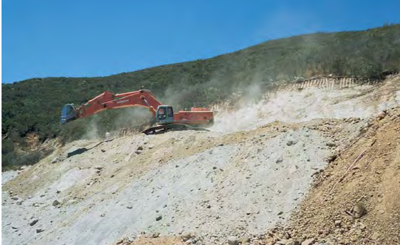
Figure 11. In July 2001, Edward Swoboda and partners used a large excavator to open-cut part of the Tourmaline Queen mine in Pala, California. Several pockets containing gem- and specimen-quality tourmaline were found after the cut was extended several meters into the pegmatite. Photo by Brendan M. Laurs.
