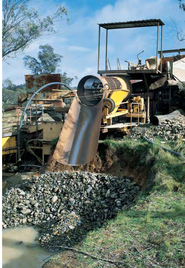
Figure 28. This equipment is used for washing the gem-bearing sediments in the Barrington Tops area of eastern Australia. Photo by Shane F. McClure.
