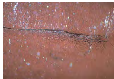
Figure 13. With 40× magnification, the crackled texture of the filler in this large fracture is easily visible among the multitude of reddish platelets and needles that cause the chatoyancy in the host iolite.
