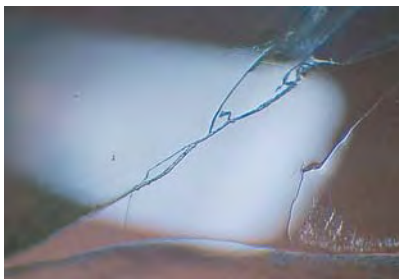
Figure 12. In reflected light, the filled fractures in this cat’s-eye iolite showed a distinctly lower relief than the rest of the stone. Magnified 24×.
