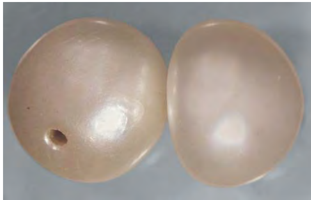
Figure 22. The 6.18 ct natural pearl on the left (shown with an untreated natural pearl on the right) proved to be coated with a resin mixed with essence d'orient. Photo by H. A. Hänni, © SSEF.
