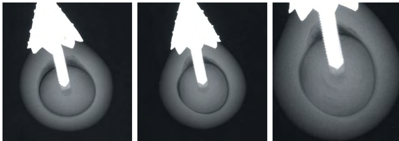
Figure 13. The first X-radiograph of the pearl in figure 12 exposed what appeared to be a spherical core that is slightly darker than the outer nacre layers (left). Another radiograph taken 90° to the first revealed a slightly asymmetrical oval outline (center) and natural features (right).
