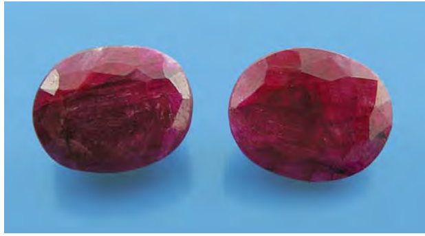
Figure 24. These two stones (9.61 and 11.40 ct) proved to be fibrolite (sillimanite) that had been dyed and impregnated to imitate ruby. Photo by S. Singbamroong, © Dubai Gemstone Laboratory.
