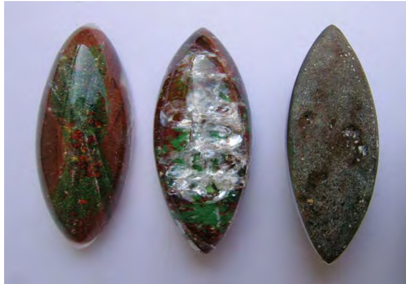
Figure 21. These rock crystal cabochons (approximately 5 cm long) from Brazil contain fake inclusions that were apparently created in a three-step process. In addition, the cabochon in the center contains reflective oval fractures that were likely induced by thermal shock. The cabochon on the right shows the base, which is covered with a mixture of glue and mineral powder. Photo by J. Hyrsl.
