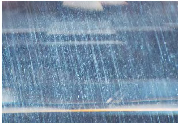
Figure 15. A dense network of parallel stringers was present in all of the tenebrescent scapolites. Photomicrograph by S. F. McClure; magnified 18x.
