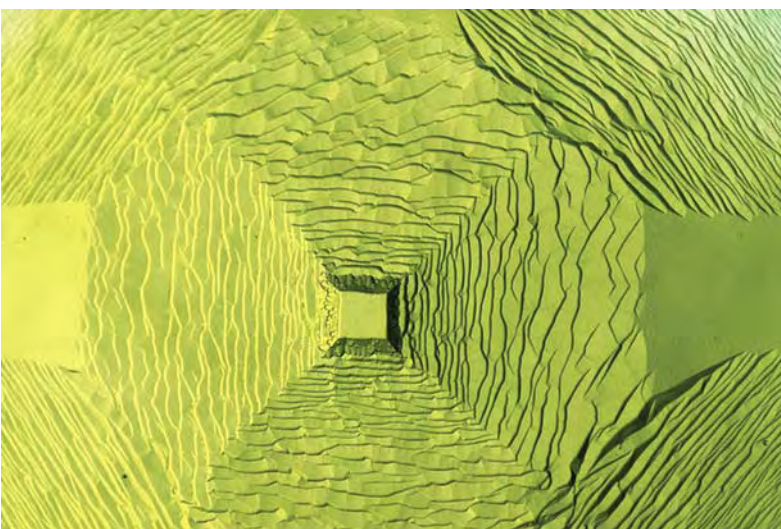
Figure 4. With a gemological microscope, portions of this high-purity CVD synthetic diamond (no. 66675) display surface growth features similar to those observed on the nitrogen-doped crystals. The apparent color is caused by the yellow substrate of HPHT synthetic diamond, which was not removed. Photomicrograph by W. Wang; image width is approximately 2.9 mm.
