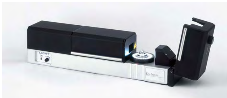
Figure 15. Once a matter of expert guesswork, the marking and dividing of rough diamonds became a far more precise and efficient process through the development of computerized scanning and measuring systems such as the Sarin DiaExpert (shown here with DiaMension hardware). Courtesy of Sarin Inc.
