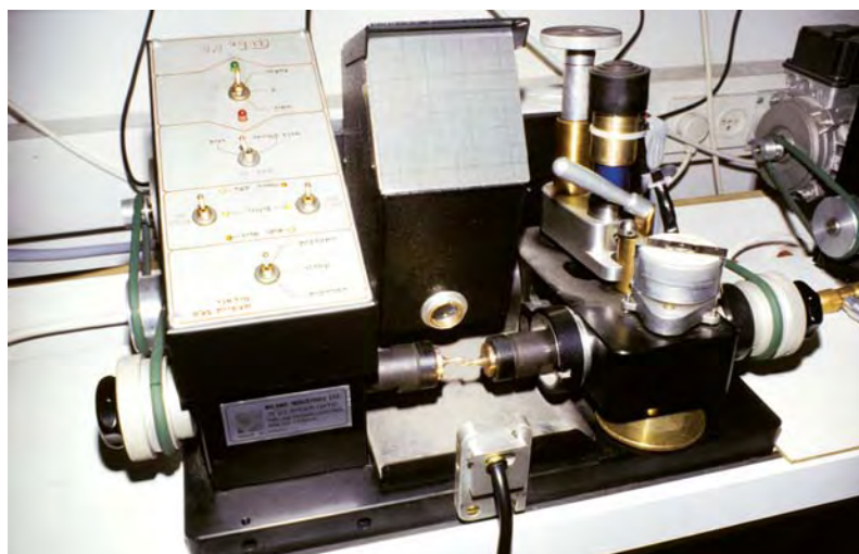
Figure 14. Bruting, or initial shaping of the rough, was once the most difficult and labor-intensive element of diamond manufacturing. The advent in the 1980s and '90s of automatic bruting machines, such as this one by Milano Industries, led to huge improvements in productivity and quality control. Photo by James E. Shigley.
