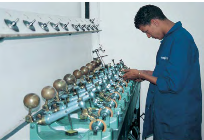
Figure 10. As African governments seek greater local benefits from their diamond resources, one primary goal is the successful development of local polishing operations. Shown here is a sawing line at the Namcot Diamonds plant in Windhoek, Namibia, operated by the Steinmetz Group. The economic viability of these operations is uncertain, since they must compete with manufacturers in countries such as India that have much lower labor costs. Photo by Brendan Laurs.
