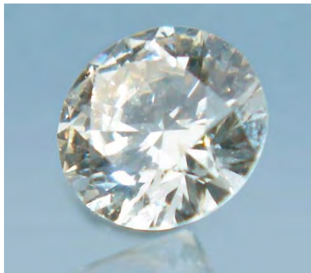
Figure 26. This 0.2 ct near-colorless CVD synthetic diamond was cut from a 1 ct block produced at a high growth rate using a focused plasma beam. Courtesy of the Carnegie Institution, Washington, DC.
