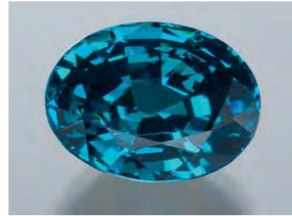
Figure 18. Resembling a high-quality zircon, this intensely colored greenish blue gem (19.66 ct) is a manufactured product, yttrium zirconium oxide.
