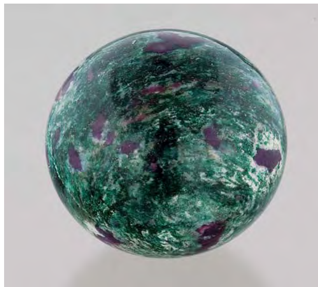
Figure 6. This sphere (5.4 cm in diameter) was cut from a rock consisting of fuchsite, corundum, and alkali feldspar. The material comes from a new deposit in Bahia, Brazil. Photo by C. D. Mengason; GIA Collection no. 32380.
