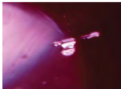
Figure 1. It is very unusual to see crystals or negative crystals such as these in a melt-grown synthetic alexandrite. Note the three minute gas bubbles hovering above the crystals. Magnified 95×.
