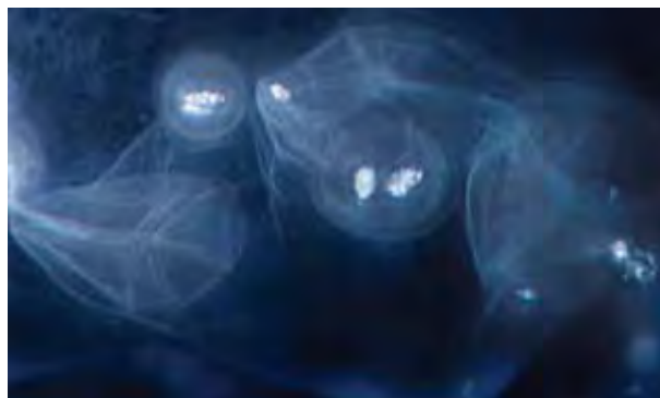
Figure 2. This cloud-like inclusion in a blue sapphire was determined to contain beryllium, but no beryllium was detected in the surrounding host. It seems very unlikely that the stone could be diffusion treated. Photomicrograph by S. F. McClure; magnified 21 \times .
