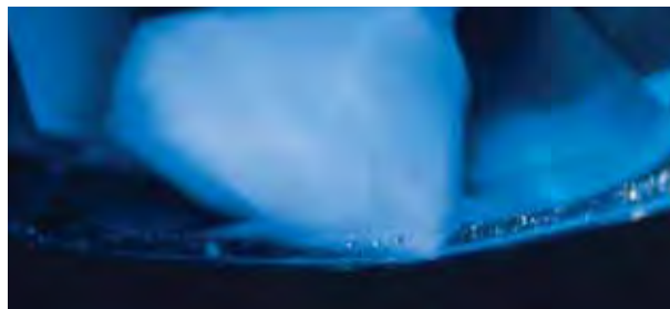
Figure 1. LA-ICP-MS analyses of this sapphire showed highly variable Be content. Photomicrograph by S. F. McClure; magnified 30x.
