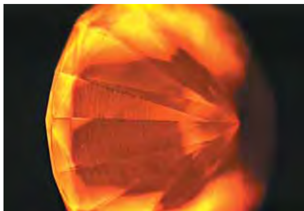
Striated orange fluorescence, seen in this DiamondView image, is characteristic of CVD synthetic diamond containing trace amounts of nitrogen. Courtesy of the DTC Research Centre.
