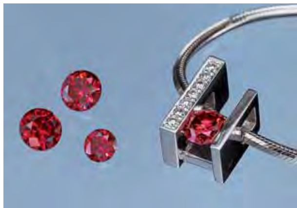
Figure 2. The color in these pink-to-red diamonds was produced by a treatment that involves HPHT annealing, irradiation, and low-pressure annealing at relatively lower temperatures. Loose stones (0.15–0.33 ct) courtesy of Lucent Diamonds; necklace courtesy of Avirom Associates. Photo © Harold & Erica Van Pelt.
