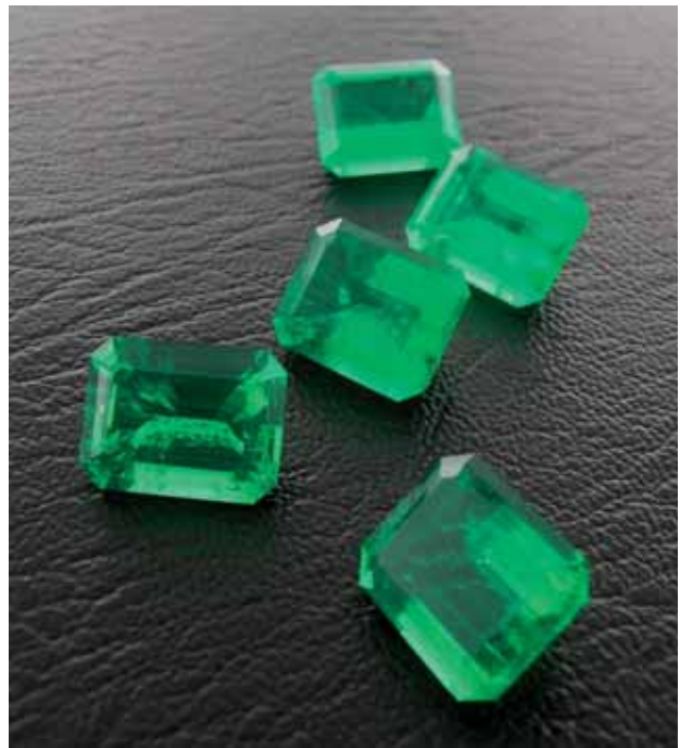
Figure 31. These large faceted samples (~13.6–16.3 ct), originally represented as Colombian emeralds, proved to be beryl triplets composed of two pieces of near-colorless beryl held together by green cement. Photo by S. Singbamroong, © Dubai Gemstone Laboratory.
