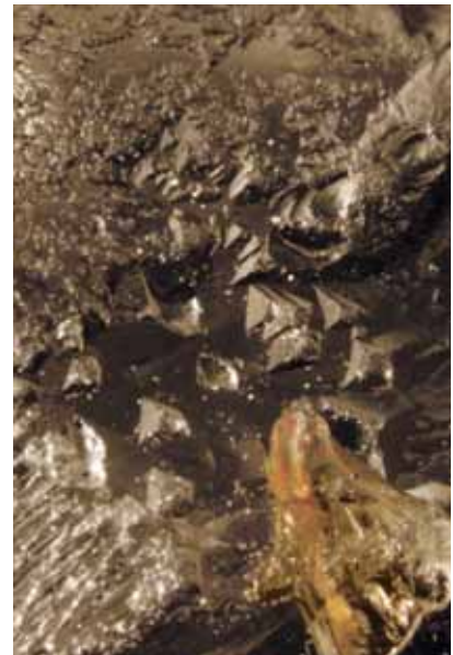
Figure 21. Trigon-like features were also present in the crystal featured in figure 19, but unlike those seen in diamond they were raised rather than indented. Width of view 7.5 mm.
