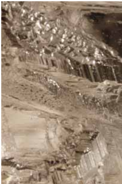
Figure 20. The crystal showed parallel, step-like growth striations, similar to what is seen on some rough diamonds. Width of view 8.9 mm.
