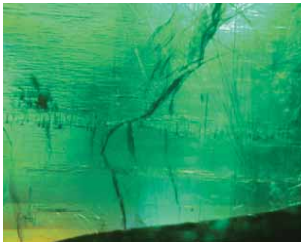
Figure 7. In this emerald, small, dark conical inclusions can be seen projecting from the parallel planes in the background, similar to nail-head spicules projecting from the seed plate in a synthetic emerald. However, the presence of abundant curved, fibrous tremolite-like inclusions indicates a natural origin: Sandawana, Zimbabwe. Photomicrograph by G. Choudhary; magnified 20 \times .
