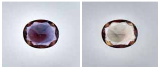
Figure 5. Violetish blue color zones are seen in the reddish purple pleochroic direction (left) of this 2.97 ct axinite from Pakistan; the colors almost disappear when the polarizer is rotated 90° (right). Gift of Herb and Monika Obodda, GIA Collection no. 37121; photos by Robert Weldon.
