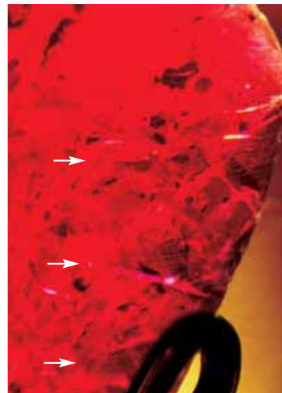
Figure 24. Curved striae were also observed when the quench-crackled synthetic ruby was viewed at 12× magnification while immersed in methylene iodide.
