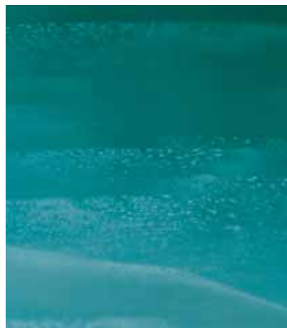
Figure 2. Growth zones parallel to the length of the aquamarine in figure 1 contained reflective crystals and films. Field of view 7.3 mm.
