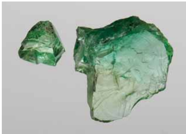
Figure 28. This Cr/V-bearing spodumene from Afghanistan (1.3 g total weight) ranges from green to light yellow-green, and a portion of the green area was separated to retain as a reference for fade-testing experiments. Sunlight exposure for three weeks did not cause discernable fading; note that the yellow-green portion on the bottom appears relatively pale colored due in part to the narrow thickness of the sample in that area. Gift of Herb and Monika Obodda, GIA Collection no. 36750; photo by Robert Weldon.
