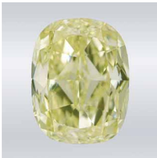
Figure 1. This 1.75 ct cushion-cut Fancy green-yellow diamond is colored mainly by Ni-related defects. Photo by Jian Xin (Jae) Liao.
