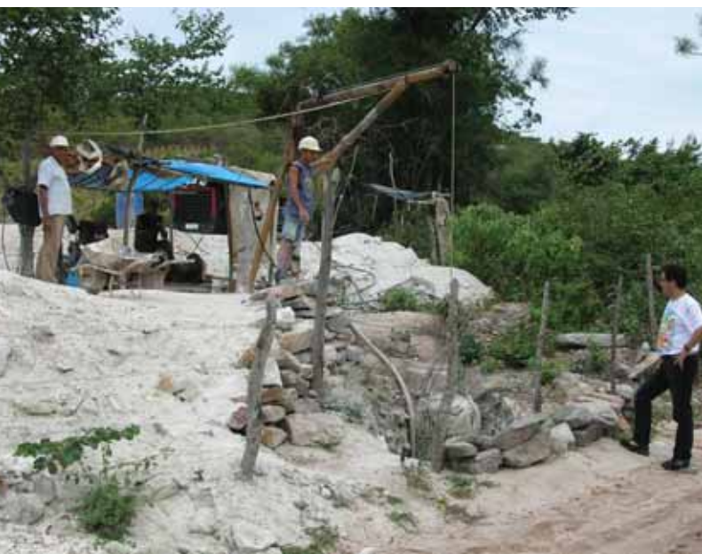
Figure 4. Located just 4 km from the original Mina da Batalha deposit, the Mineração Batalha mine was being explored by a shaft 20 m deep in April 2007. Photo by M. Furuya.
