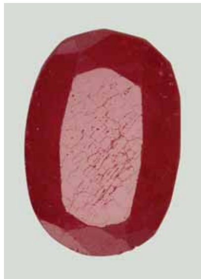
Figure 22. This 12.84 ct specimen (15.95 × 10.80 × 7.74 mm) proved to be a quench-crackled, glass-filled synthetic ruby.
