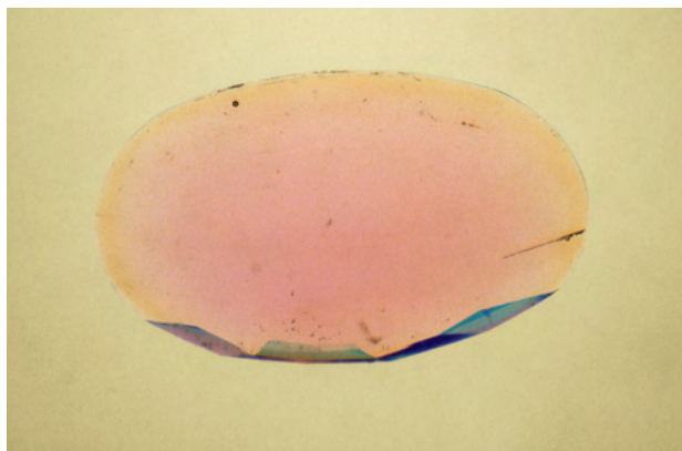
Figure 9. A shallow surface-related orange rim around a pink core is diagnostic of some Be-diffused sapphires. Photomicrograph by S. F. McClure; magnified 10x.
