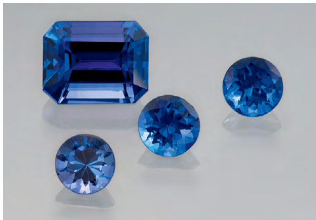
Figure 22. Tanzanite coated with a cobalt-colored material was of great concern for a brief time. All of these tanzanites (0.50–3.01 ct) were coated, but the one on the lower left was repolished to give an idea of the original (paler) color. Courtesy of Fine Gems International; photo by Roger Mathis, ©Robert E. Kane.
