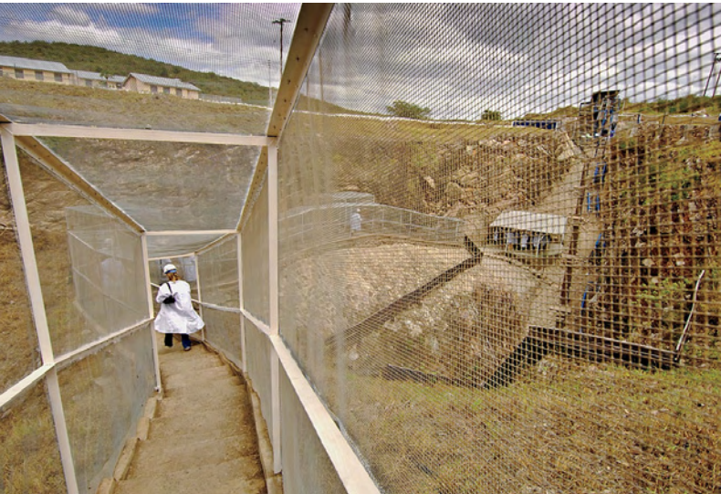
Figure 10. TanzaniteOne, formerly Afgem, is licensed to mine tanzanite at Block C in Merelani, Tanzania. This high-security screen enclosure (designed to prevent theft) guides miners to different shafts at the mine. Photo by R. Weldon.
