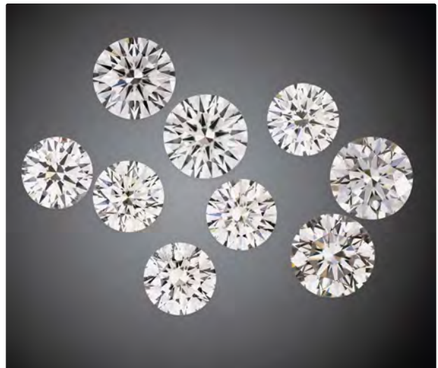
Figure 1. Colorless gem-quality CVD-grown synthetic diamonds such as these (0.22–0.31 ct) are now commercially available, making proper identification important. Photo by Robert Weldon.
