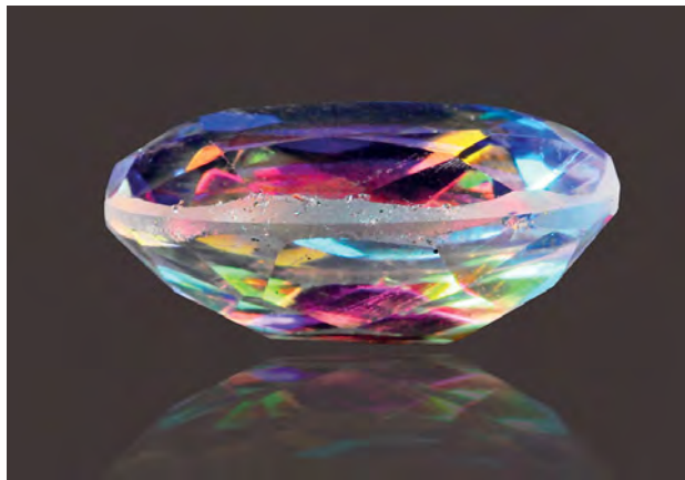
Figure 48. The two halves of this colorful glass triplet (12.28 × 17.33 × 7.92 mm) are easily visible to the naked eye. The junction between them is seen within the frosted girdle. Photo by O. Segura.
