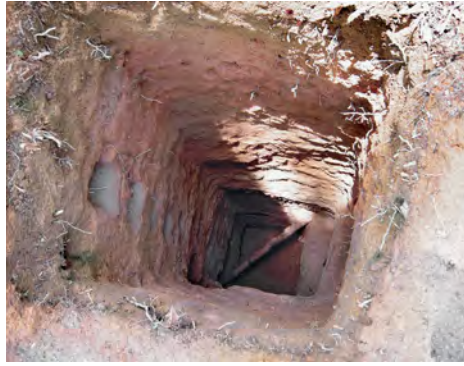
Figure 6. At the Thanh Hoa deposits, ropes are used to hoist aquamarine-bearing material from shafts (left). Some of the shafts reach depths of ~15 m (right). Photos by D. Blauwet.
