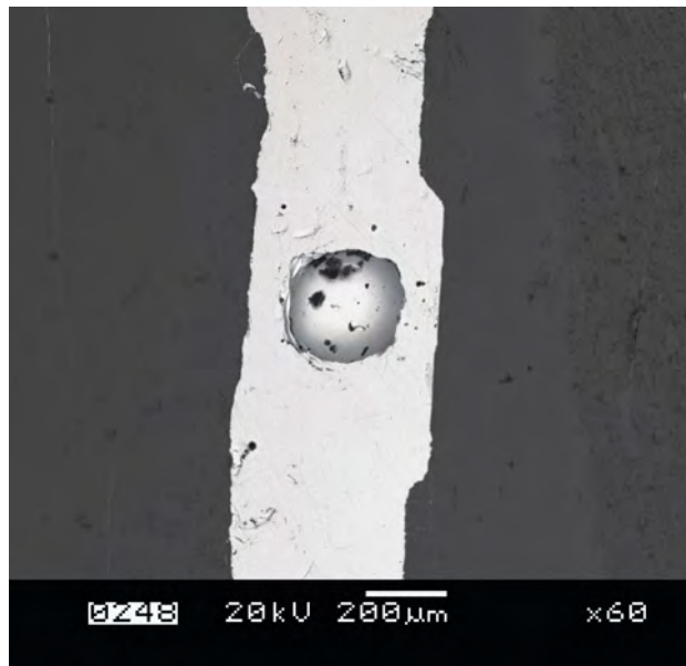
Figure 47. In this backscattered electron micrograph, the transparent layer in the black star sapphire shows a light tone indicative of a high atomic number, consistent with a high lead content. A surface-reaching bubble is seen in the center; note that the two sides of the fracture do not correspond in shape. Image by E. Fritsch.
