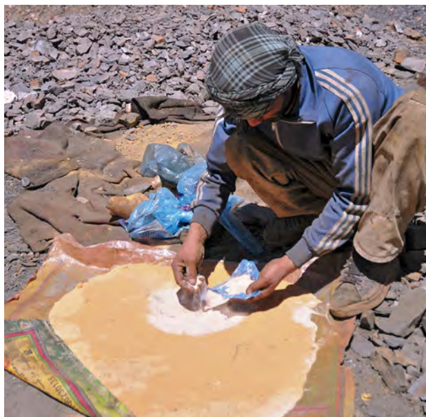
Figure 11. Afghan emerald miners mix fertilizer with old Soviet military explosives for blasting purposes, which often damages the fragile crystals. Photo by V. Pardieu.
