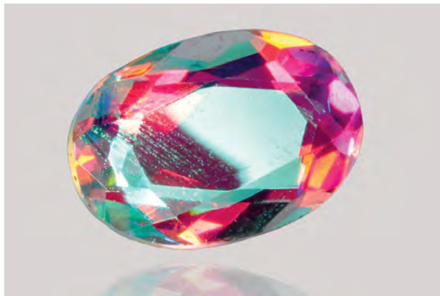
Figure 49. Viewed face up, the internal iridescent layer in the glass triplet reflects scratches on the table. Photo by O. Segura.
