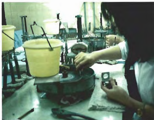
Figure 1. Diamonds are being cut in Foshan, China, using a variation of the jam peg method. Photo by Robert C. Kammerling.
