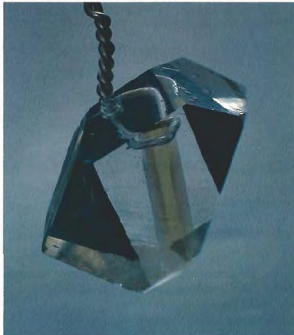
Figure 5. When a Brazil law-twinned amethyst seed plate oriented near-perpendicular to the c -axis direction was used, the resulting 16-mm-long synthetic quartz crystal took a form more closely resembling that of natural quartz. Heat generated during the growth process converted the amethyst seed to citrine. Irradiation would restore the purple color. Photo by Robert Weldon.
