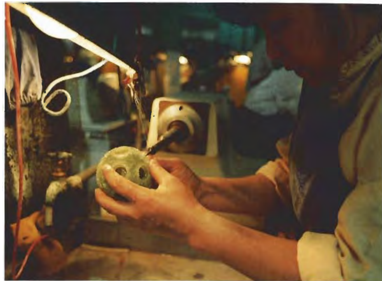
Figure 11. This Chinese artisan uses a lathe drill to fashion a “jade carving ball” that had the appearance of serpentine. Photo by Robert C. Kammerling.
