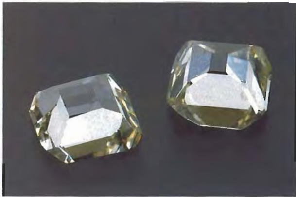
Figure 1. These two near-colorless synthetic diamond crystals, grown by the new GE process, were loaned to GIA by GE Superabrasives in Worthington, Ohio. Some crystal faces of these 0.91- and 1.04-ct (respectively) cuboctahedral crystals have been polished. Photo by Maha DeMaggio.
