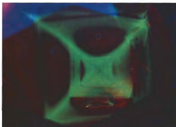
Figure 8. The crown facets of the 0.55-ct red synthetic diamond reveal an uneven, intense fluorescence to short-wave U.V. radiation. The combined square- and cross-shaped pattern of green fluorescence corresponds to the light yellow zones in the diamond; the moderate reddish orange fluorescence to the red areas in the stone. Photomicrograph by John I. Koivula; magnified 5 \times .
