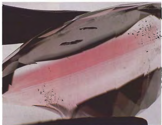
Figure 16. Examination at 10 \times magnification reveals that the pink color of the stone in figure 15 is confined to densely packed bands.
