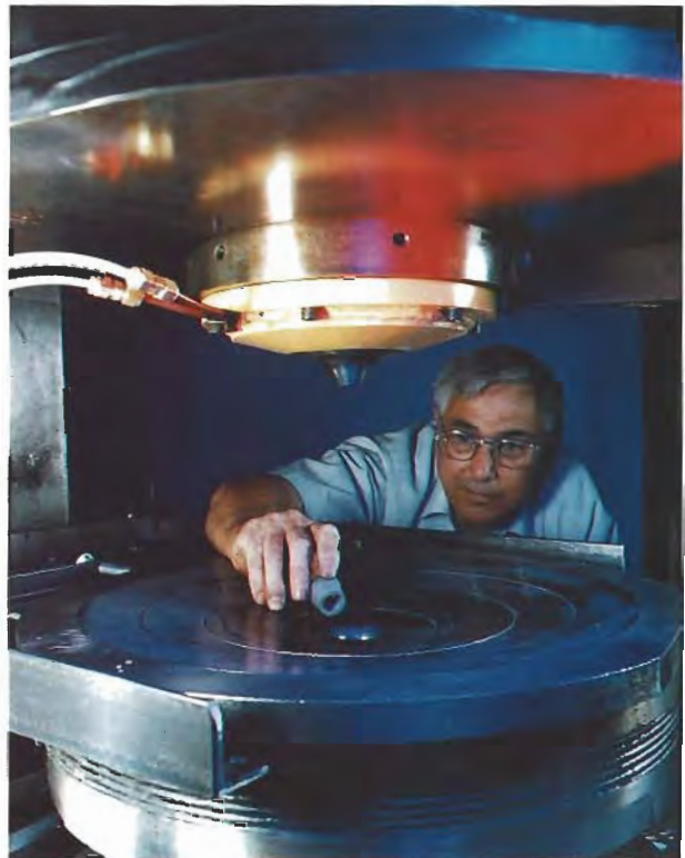
Figure 2. A General Electric scientist prepares the high temperature/high pressure "belt" apparatus for growing synthetic diamond crystals. Photo courtesy of General Electric.
