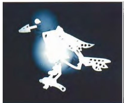
Figure 13. An X-radiograph of the brooch in figure 12 proves that the pearl is cultured and has two separate beads.
