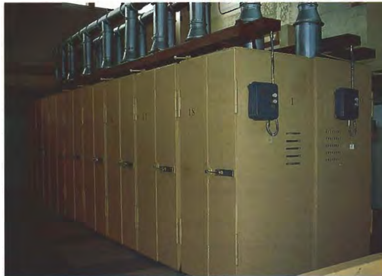
Figure 17. Each of the metal containment safes in the new Taurus joint-venture facility in Novosibirsk, Siberia, contains a hydrothermal autoclave. Most of the production is synthetic emerald, but there are also smaller quantities of synthetic ruby. Photo by Robert C. Kammerling.
