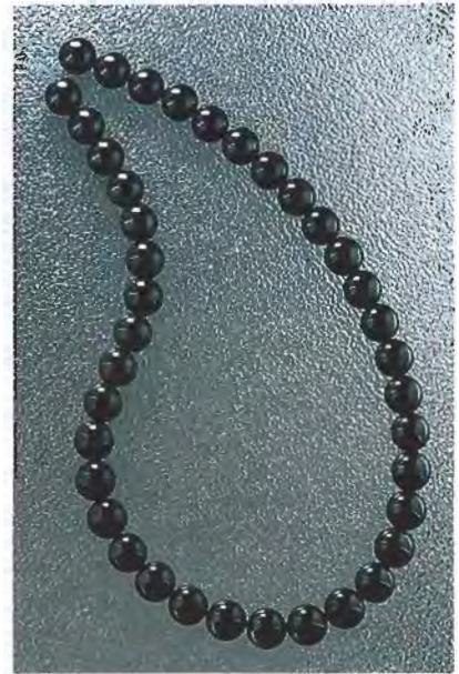
Figure 5. Although these 10-mm opaque black beads were purchased as jadeite from Arizona, extensive testing revealed that they are actually ferrohornblende.
