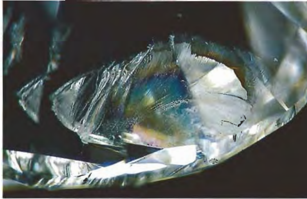
Figure 36. One method for determining whether a suspect fracture is filled is to see if water can be drawn into it. On the left is an unfilled fracture with natural iridescence. On the right is the same fracture after water was applied to its entry point at the diamond's surface; note the decrease in relief of the fracture, as well as the bubbles apparent in the water that was drawn into the break. With the microscope, one can actually see the bubbles move. Photomicrographs by Shane F. McClure; magnified 33 \times .
