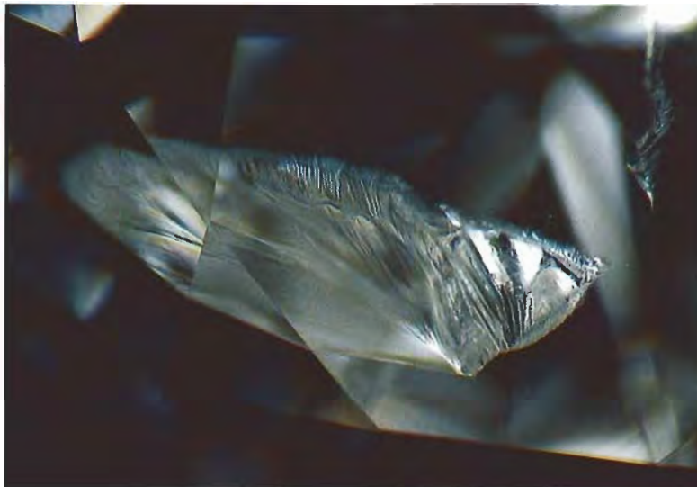
Figure 40. The high relief and feathery appearance typical of many unfilled breaks have not been noted in any of the fracture-filled diamonds examined by the authors. Photomicrograph by Shane F. McClure; magnified 33 \times .
