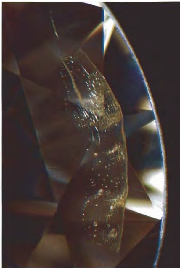
Figure 17. A crackled texture was noted in some of the thicker areas of filling in Yehuda-treated diamonds. Photomicrograph by Shane F. McClure; magnified 40 \times .
