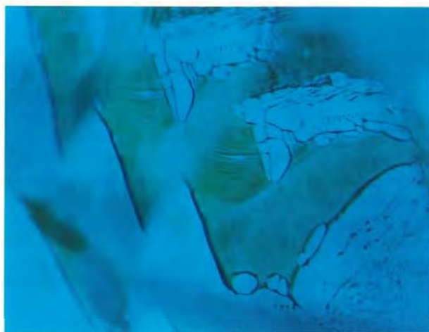
Figure 16. Primary flux inclusions form phantom structures in this synthetic phenakite manufactured in Russia. Photomicrograph by John I. Koivula; magnified 25 \times .
