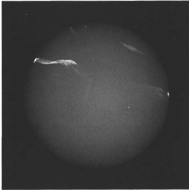
Figure 22. This X-radiograph of a fracture-filled diamond illustrates the extremes of filler visibility by this testing technique. Obvious white areas are evident on the perimeter of the stone, while the L-shaped filled break in the center is barely discernible. X-radiograph by Karin Hurwit.
