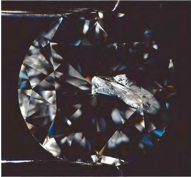
Figure 3. This 0.30-ct diamond, which had highly visible breaks before fracture filling (left), showed significant improvement in apparent clarity—from I_3 to I_1 —after treatment by Goldman Oved (right). Photomicrographs by Shane F. McClure.
