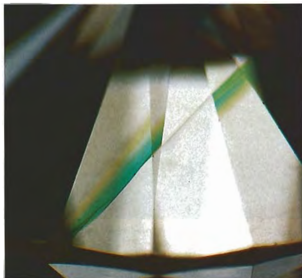
Figure 5. Brightfield flash-effect colors in the newest generation of Yehuda-treated diamonds range from bluish green to greenish yellow. Photomicrograph by Shane F. McClure; magnified 28 \times .
