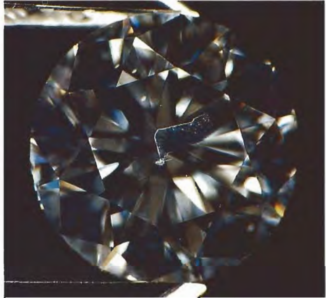
Figure 3. This 0.30-ct diamond, which had highly visible breaks before fracture filling (left), showed significant improvement in apparent clarity—from I_3 to I_1 —after treatment by Goldman Oved (right). Photomicrographs by Shane F. McClure.
