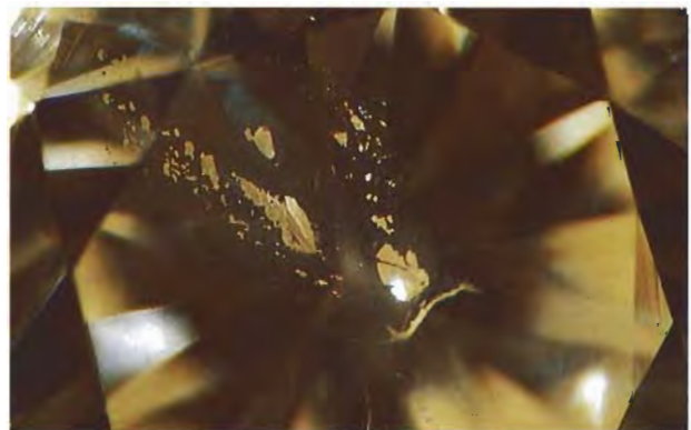
Figure 15. Some of the Goldman Oved-treated diamonds displayed relatively large gas bubbles in their fillings. Photomicrograph by Shane F. McClure; magnified 33 \times .
