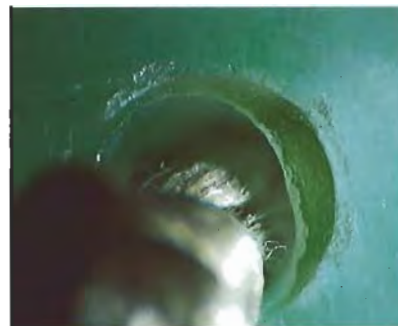
Figure 7. Residue of the polymer material with which this jadeite bead was impregnated is evident in its drill hole. Magnified 28x.
