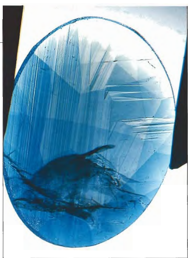
Figure 10. The internal growth structures seen in many of the sapphires provided enough information to enable the senior author to extrapolate the original crystal habit. This 0.44-ct Vietnamese sapphire shows a combination of crystal planes, composed of: basal pinacoid c (0001), the roughly horizontal growth planes; connected to a more subordinate series of dipyrmaid n ( 22\bar{4}3 ) crystal planes, creating an angle of 118.8^\circ with the basal growth planes; and dominant dipyrmaid z ( 22\bar{4}1 ) crystal planes, the nearly vertical growth planes, creating an angle of 100.4^\circ with the basal growth planes. Rotating this stone about the vertical axis through 30^\circ , a combination of c (0001) and r ( 10\bar{1}1 ) crystal planes were visible, creating an angle of 122.4^\circ . This information permits a crystal habit of c , r , n , and z to be assumed for the original crystal (also refer to figure 11b). Immersion, view perpendicular to the c -axis, transmitted illumination, magnified 15 \times .
