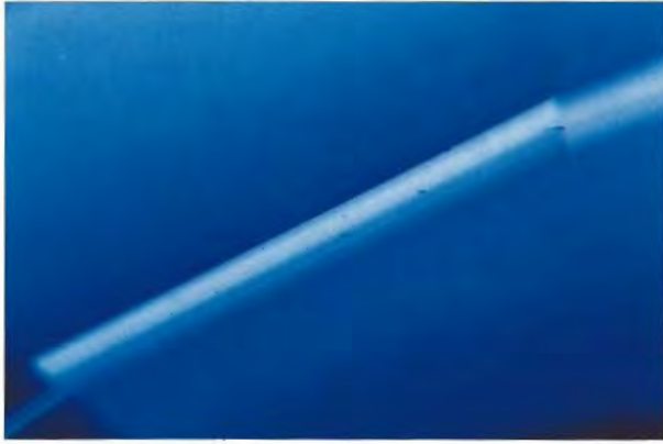
Figure 13. Strong, sharply bordered blue color bands alternating with narrow colorless bands was one type of distinctive color zoning noted in the sapphires from southern Vietnam. Photomicrograph by Dr. Eduard J. Gübelin; magnified 50 \times .
