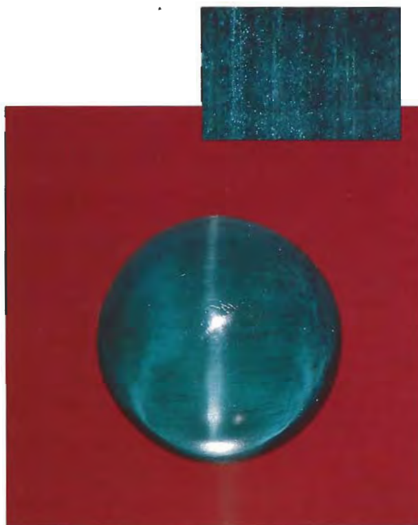
Figure 3. Note the pronounced eye and unusual color of this 11.45-ct blue-green apatite cabochon, reportedly from Madagascar. Short, barely visible white needles cause the chatoyancy (inset). Photo by Shane F. McClure; photomicrograph by John I. Koivula, magnified 50×.
