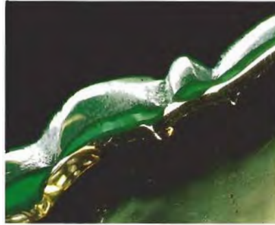
Figure 11. The thin edge of the hollowed-out carving shown in figure 10 was visible between the mounting and the bottom of the stone. The plastic filler (which is actually colorless, but appears green in this photo because of the jadeite shell) can be seen under the edge of the jadeite, following the contours of the carving. Magnified 13×.
