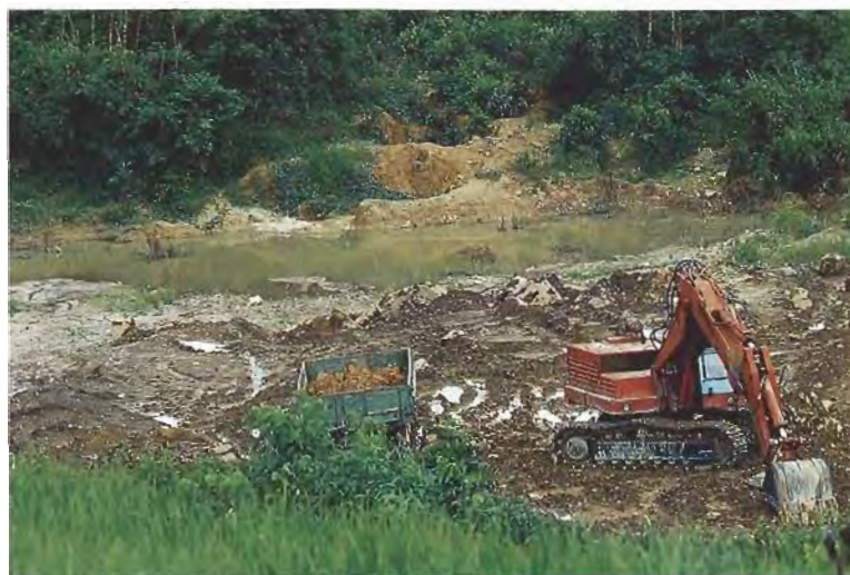
Figure 7. At Di Linh, in Lam Dong Province, the joint venture Vinagemco uses a backhoe to remove the overburden and reach the gem gravels. A dump truck then carries the gravels to a nearby washing plant. Photo by K. V. Scarratt.
