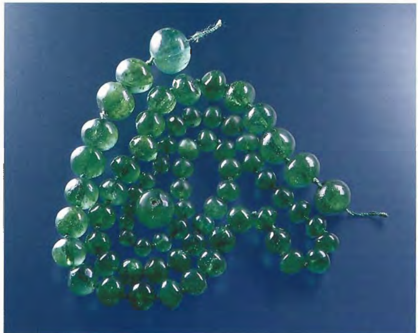
Figure 7. This imitation emerald necklace consists of 5.10–16.0 mm natural beryl beads that have been coated with a green plastic.
