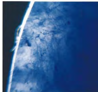
Figure 16. Magnification of one of the scarabs in figure 15 reveals dye concentrations in the fractures, which are responsible for the lapis-like color. Magnified 10×.
