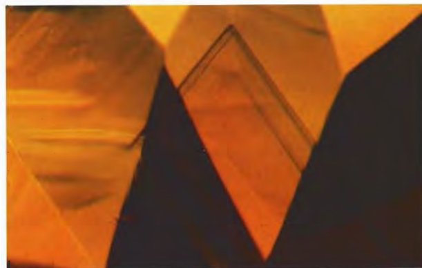
Figure 13. The growth zoning seen here in a 15.67-ct dark orangy brown garnet from Mali appears to parallel trapezohedral growth faces. Photomicrograph by John I. Koivula; magnified 20 \times .
