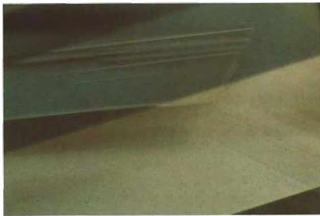
Figure 12. Straight growth zoning parallel to two dodecahedral faces was commonly seen in the test sample of grossular-andradite garnet from Mali (left). This feature appears particularly sharp when viewed between crossed polarizers (right). Photomicrographs by John I. Koivula; magnified 20 \times .
