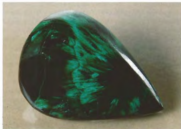
Figure 17. Opticon, or a similar synthetic resin, was used to impregnate this 17.19-ct fibrous-appearing malachite. Photo by Maha DeMaggio.
