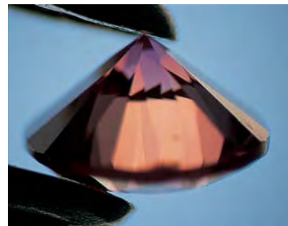
Figure 5. Irradiation with an electron beam created the concentrated purple zone seen at the culet. The combination of this purple zone and the light yellow bodycolor gives rise to the overall “peach” color seen here. Magnified 25x.
