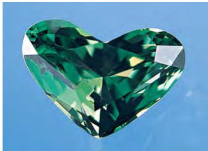
Figure 3. This 3.65 ct dark green chrysoberyl is colored by vanadium. It reportedly came from Tunduru, Tanzania.
