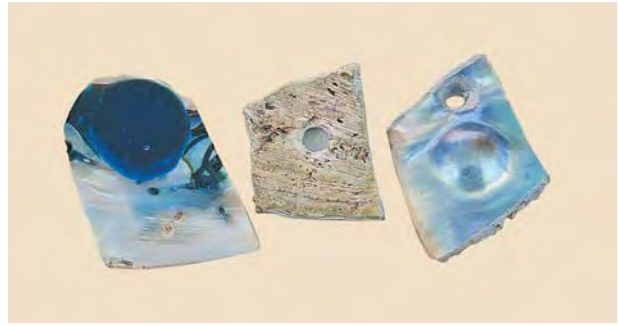
Figure 11. The two unprocessed, unpolished samples on the right were still in the shell with the hemispherical bead nuclei intact (note that the intensity of the colors is similar to the assembled product). The center sample is positioned face-down, to show the rough surface of the outer shell. The sample on the left (also face-down) had been separated from the outer shell, filled with blue polymer, and partially polished. Courtesy of Empress Abalone Ltd.; photo by Maha DeMaggio.
