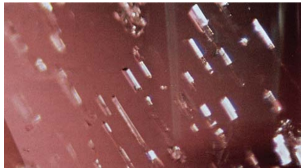
Figure 6. Healed fractures in the taaffeite samples typically appeared as groups of negative crystals with multiphase fillings. Sample G; magnified 200 \times .
