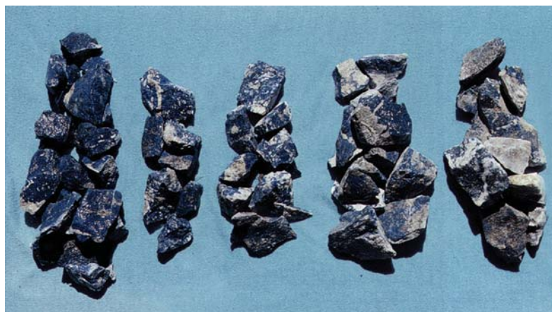
Figure 12. These samples represent the graded material studied by the authors. From left to right: first-quality (150 g), second-quality (100 g), third-quality (100 g), fourth-quality (170 g), and reject material (180 g).
