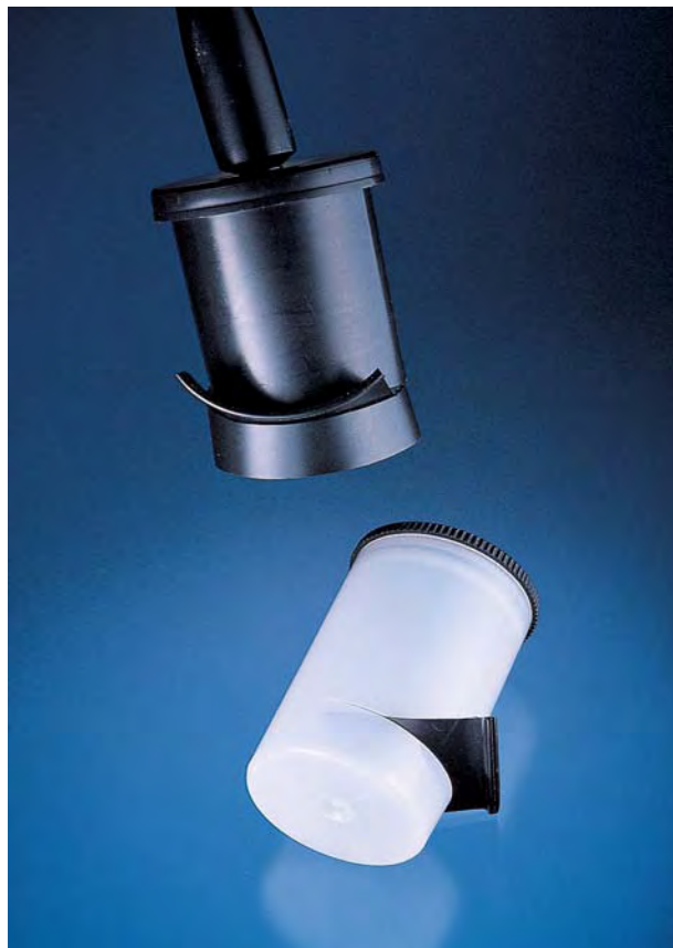
Figure 30. Simple light shields for blocking hot spots produced by fiber-optic illuminators can be manufactured from plastic film canisters. The translucent white light shield provides diffused fiber-optic illumination, while the one constructed from an opaque black film canister provides intense direct fiber-optic lighting. Photo by Maha Tannous.
