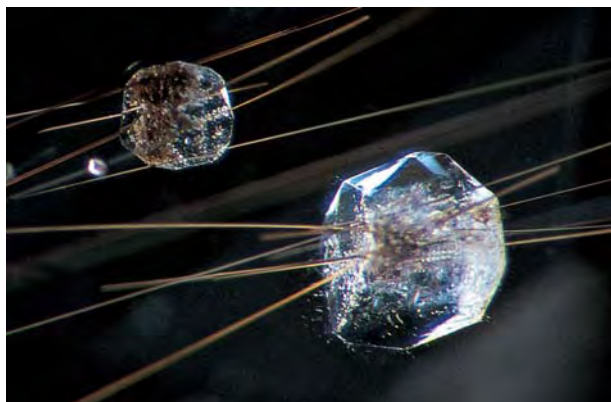
Figure 29. An even more effective method of controlling hot spots is to block the light source rather than moving the subject. This is done by placing a thin strip of opaque black paper in front of the area of the light that is producing the hot spot. Compare this image to the one on the left in figure 28 (with the hot spot): The position of the inclusions in this photo is an exact match. Magnified 15×.
