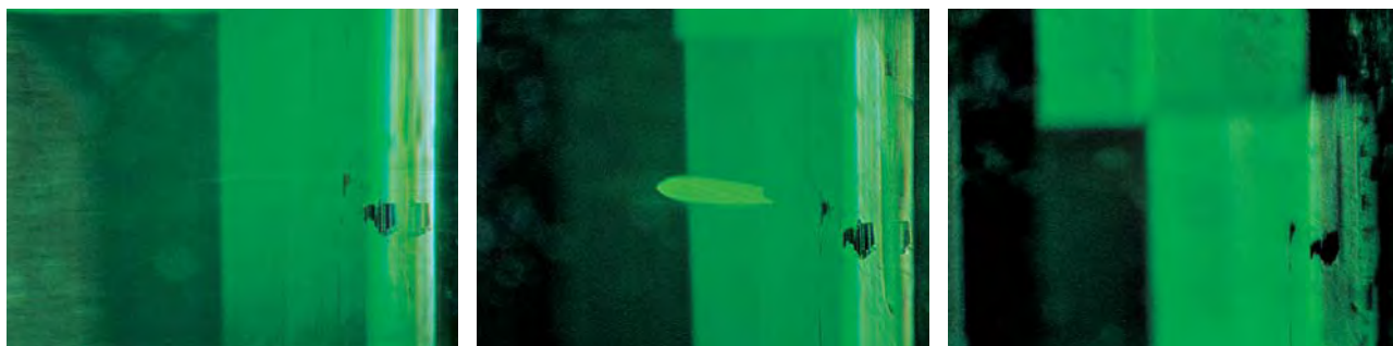
Figure 32. Another illustration of the importance of illumination angle is found in this darkfield sequence of three photomicrographs, each of which represents a slight tilting of the emerald relative to the light. In the image on the left, a filled crack is virtually invisible when viewed parallel to its plane. In the center view, as the stone is slightly tilted the air trapped inside the filler becomes visible, revealing the presence of the filling itself. Tilting the emerald only a little further causes the reflection from the trapped air in the filled crack to virtually disappear again. Magnified 15 \times .
