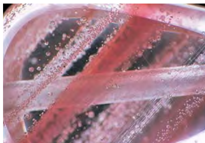
Figure 10. Planes of spherical gas bubbles and irregular pink and colorless banding were clearly visible in this glass bead. Magnified 15 \times .
