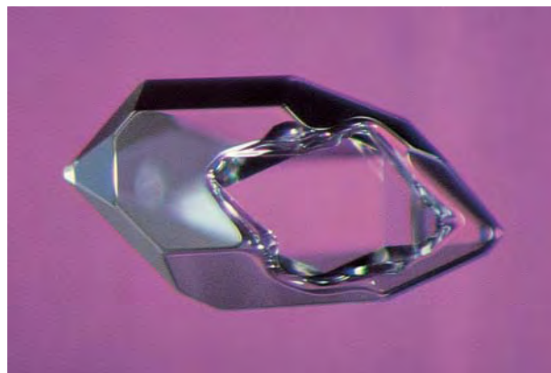
Figure 16. Transmitted light was used to illuminate this relatively large negative crystal in an amethyst from Mexico. Magnified 10 \times .
