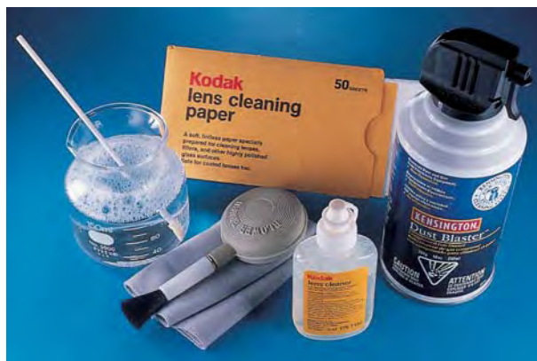
Figure 5. Items for cleaning optical equipment as well as gems, such as compressed air, a camel's-hair blower brush, cleaning fluids, a gem cloth, and lens paper, should always be kept close at hand while doing gemological photomicrography. Photo by Maha Tannous.
