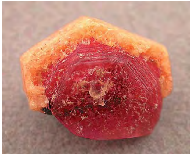
Figure 10. This crystal of Cs-“beryl” displays a pale pinkish orange overgrowth over a purplish pink core. Electron-microprobe analyses showed slightly more Cs in the rim. Courtesy of Laurent Thomas; photo by W. Simmons.
