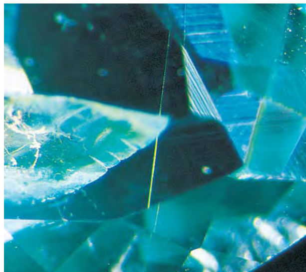
Figure 2. This needle-like channel in the faceted grandidierite from Sri Lanka is filled with a polycrystalline material. Unfortunately, there was not a sufficient amount of this polycrystalline material to identify it by Raman analysis. Note also, to the left, one of two fractures seen in the stone. Photomicrograph by H. A. Hänni; magnified 40 \times .
