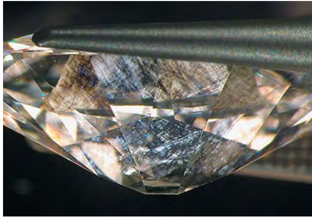
Figure 22. In cross-polarized light, a tatami strain pattern was observed in this 3.54 ct type IaB diamond with a low nitrogen concentration. Photomicrograph by J.-P. Chalain, © SSEF.
