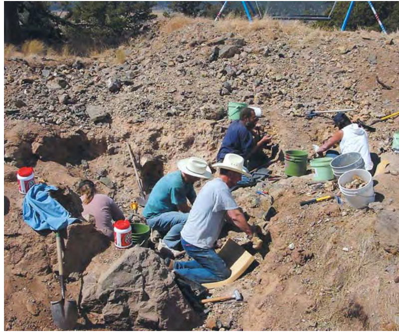
Figure 14. At Juniper Ridge, in southern Oregon, fire opal is mined from a shallow pit. Here, fee diggers are extracting opal with simple hand tools. Photo by Ken Newnham.
