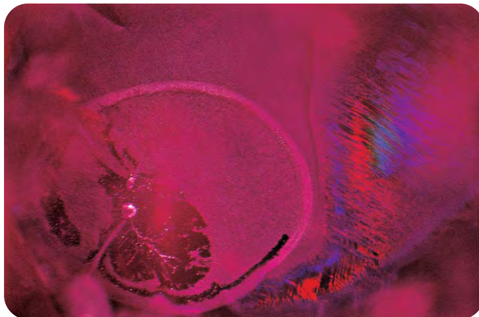
Figure 1. This decrepitation halo surrounding a fluid inclusion in a natural, untreated Thai ruby was captured on film using a combination of darkfield and fiber-optic illumination. A Polaroid analyzer was also used to eliminate image doubling, thereby providing a sharper photo. Magnified 45x.
