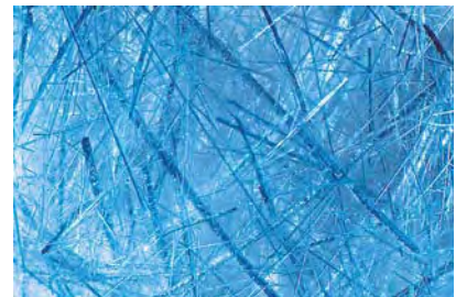
Figure 14. Thick to thin in diameter, and randomly scattered, these deep grayish blue indicolite inclusions are responsible for the apparent blue color of their quartz host. Magnified 10×.
