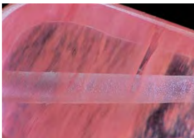
Figure 11. Somewhat reflective “copper”-colored clouds of unknown composition were also common in these glass beads. Magnified 15 \times .
