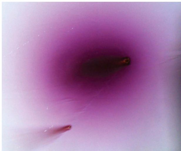
Figure 5. Pink-colored growth tubes in Cu-bearing tourmalines have a wide range of diameters; only the largest will be clearly visible without magnification. Photomicrograph by J. I. Koivula; field of view 2.9 mm.
