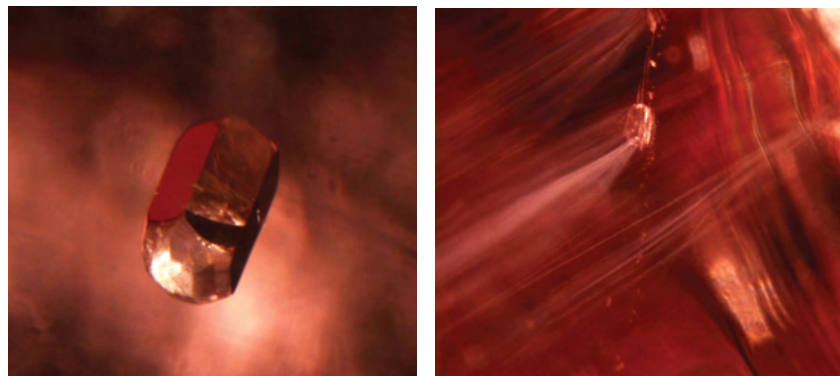
Figure 10. Among the inclusions observed in the rough spinels were a fine euhedral crystal (left, magnified 75×) and crystals with white particulate trails forming "comet tails" (right, magnified 35×).
