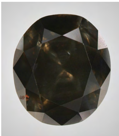
Figure 3. This 2.46 ct Fancy black diamond contained dark sectorial clouds as well as assemblages of mineral inclusions, which formed in etch channels.
