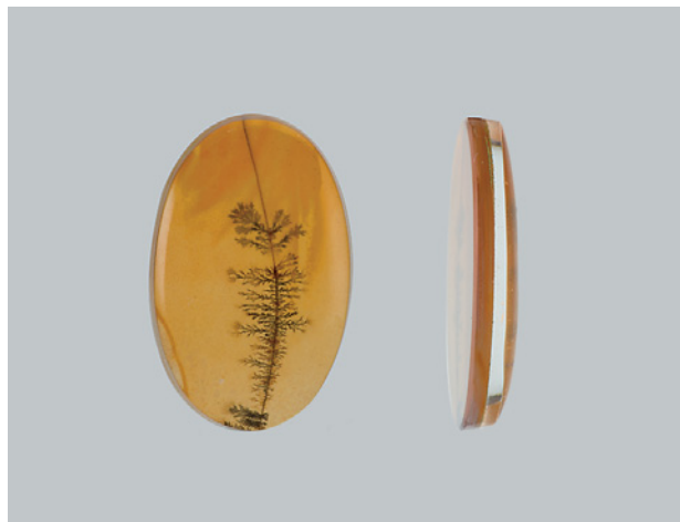
Figure 16. The profile view of this 16 × 25 mm agate doublet reveals its quartz cap. Composite photo by Robert Weldon.
