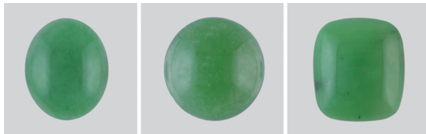
Figure 11. These three similar-looking stones were identified (left to right) as jadeite (23.90 ct), omphacite (8.12 ct), and hydrogrossular (13.90 ct).
