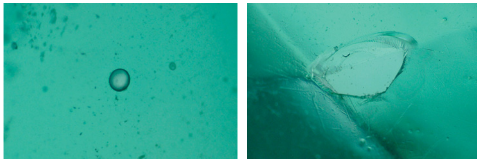
Figure 39. Gas bubbles were common at or near the surface of the briolette, suggesting a coating (left, magnified 60×). Chipped areas of coating around the drill hole revealed the colorless quartz underneath (right, magnified 45×). Photomicrographs by G. Choudhary.
