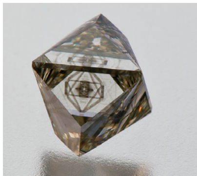
Figure 7. This 1.05 ct Fancy gray-greenish yellow diamond contains a cloud with an octahedral structure that matches that of the polished faces.
