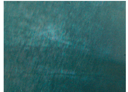
Figure 17. Dense stringer-like dislocations throughout the synthetic star spinel, viewed here at 60× magnification, produced the asterism.
