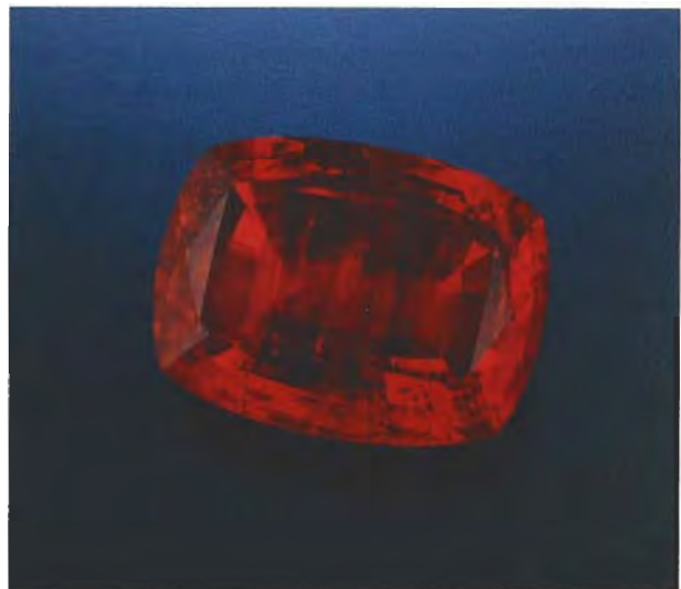
Figure 2. Large Knischka flux-grown synthetic crystals, like the one from which this 52.06-ct cushion cut was faceted, have been grown recently. Stone courtesy of P. O. Knischka; photo by Shane F. McClure.
