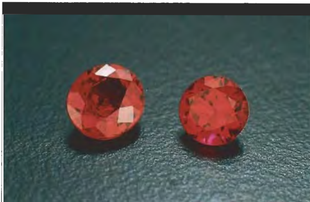
Figure 10. XRF has been used to separate natural (left) from synthetic (right) rubies on the basis of their trace elements. However, the gemologist must be careful of the artifacts in the XRF spectra when making a determination. For example, the XRF spectrum of a flame-fusion synthetic ruby shows (at the far right) a band at the position expected for gallium, an element presumed to be typical of natural rubies, and (closest to the first, on the left) a band at the exact position expected for iron, an element generally not present in flame-fusion synthetic rubies. Both peaks are actually due to diffraction, not gallium or iron. Photos by Robert Weldon.
