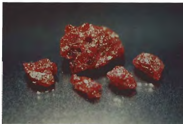
Figure 19. These rough clusters (the largest is 30 ct) show the aggregate-like nature of this new synthetic ruby, which is reportedly manufactured in the USSR. Photo courtesy of Dr. Ulrich Henn and Prof. Dr. Hermann Bank, Deutsche Stiftung Edelsteinforschung.
