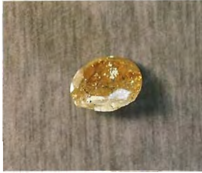
Figure 3. The remaining portion of a 3.22-ct flawless fancy yellow diamond that shattered on the wheel during a minor repair to its cut is now almost worthless.
