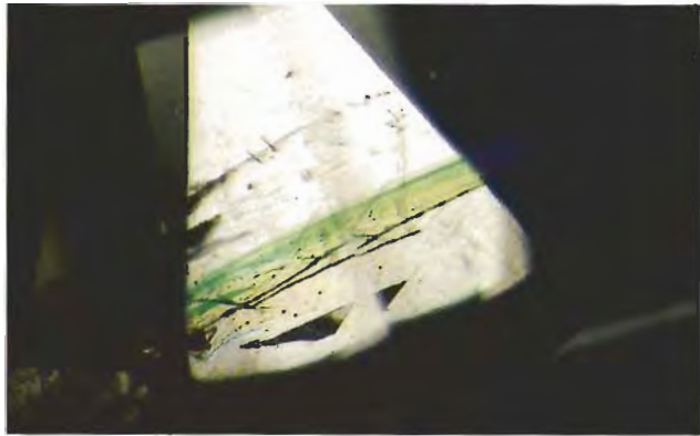
Figure 11. Some diamonds with filled breaks have been observed to exhibit previously unreported pinkish purple (left) and yellowish green (right) "flash effects." Photomicrographs by John I. Koivula; magnified 15×.
