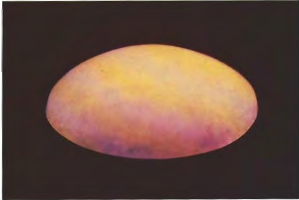
Figure 14. The strong orange fluorescence to long-wave U.V. radiation of this lavender jadeite indicates that the color is a result of dye treatment. Photo by Tino Hammid.
