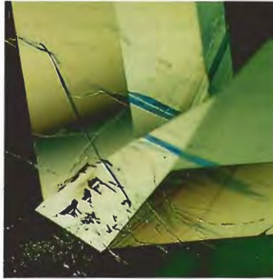
Figure 6. Orange (left) and blue (right) flashes similar to those observed in "filled" diamonds were readily apparent in the surface-reaching fractures of this emerald. Magnified 15 \times .
