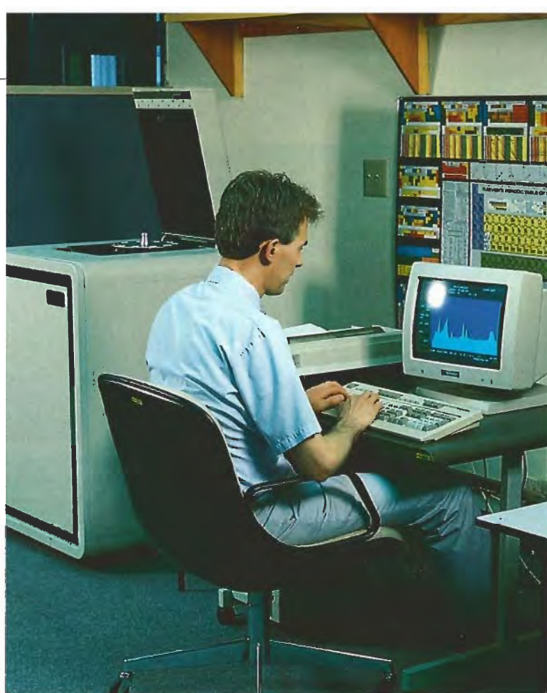
Figure 8. XRF technology was used throughout the 1980s by a number of advanced gem testing laboratories. The GIA Research Department found this Tracor X-ray Spectrace 5000 energy dispersive X-ray fluorescence (XRF) spectrometer to be useful, for example, in the separation of freshwater from saltwater pearls (see below) and untreated from fracture-filled diamonds. Photo by Robert Weldon.
