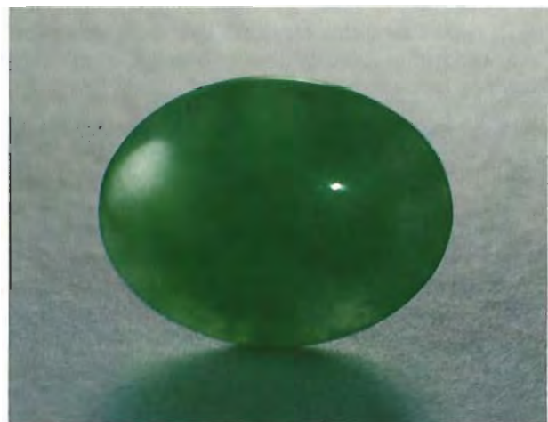
Figure 4. Selective dyeing makes this 11.54-ct (19.60 × 15.03 × 5.76 mm) quartzite cabochon an effective imitation of mottled jadeite. Photo by Robert Weldon.
