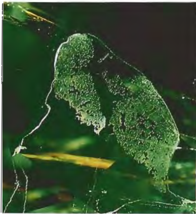
Figure 7. Trapped gas bubbles are evident in this area of the fracture where the filling is incomplete. Magnified 20 \times .
