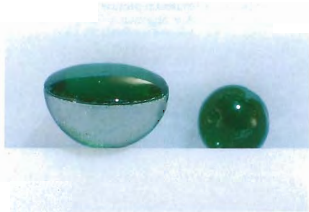
Figure 1. When viewed face-up (right), these beryl triplets appear green; examined from the side (left), the true colorless nature of the domes becomes apparent. Photo by Robert Weldon.
