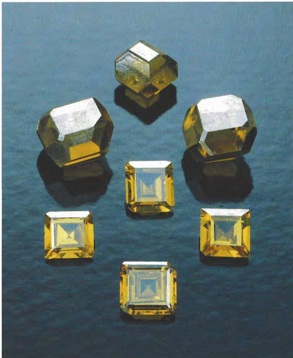
Figure 10. For the first time in the 1980s, gem-quality synthetic diamonds were sold commercially, although not generally for gem use and only in various shades of yellow. These synthetic diamond crystals (0.63–1.07 ct), and the ones from which their faceted counterparts (0.16–0.24 ct) were cut, were obtained by GIA from Sumitomo Electric Industries. Photo © Tino Hammid.
