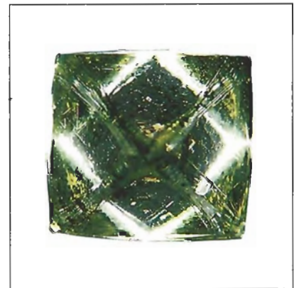
Figure 7. This 7.56-ct (12.33 \times 12.17 \times 12.13 mm) octahedral diamond is an example of rough with green surface color.
