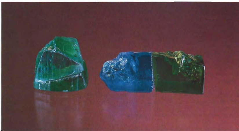
Figure 16. For the heat-treatment experiments, crystals were cut in half, with one half used as the control specimen and the other heated to 650°C. Here the halves of two specimens show, on the left (total weight, 3.64 ct), that there was no change in the “pure” green material and, on the right (total weight, 5.94 ct), the change produced in material that was originally brownish green. Photo by Shane F. McClure.
