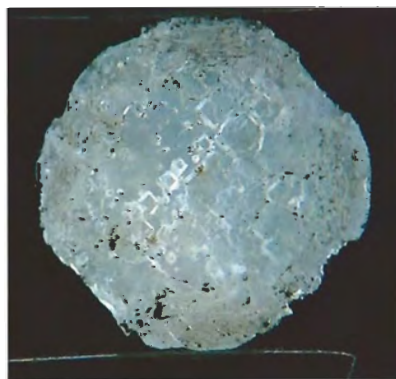
Figure 5. Prominent etch marks can be seen on the surface of this 1-ct diamond that was damaged in a fire. Magnified 18 \times .
