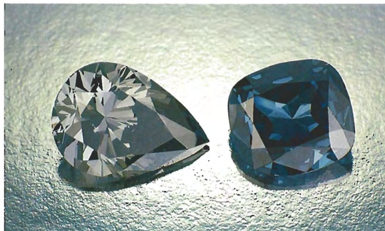
Figure 1. The crystals from which this 4.15-ct fancy bluish gray pear shape (stone A) and 3.06-ct fancy dark blue cushion modified brilliant (stone B) were fashioned were not electrically conductive, although the faceted stones are. Diamonds courtesy of Mr. R. Vainer and Mr. Th. Horovitz; photo by Robert Weldon.
