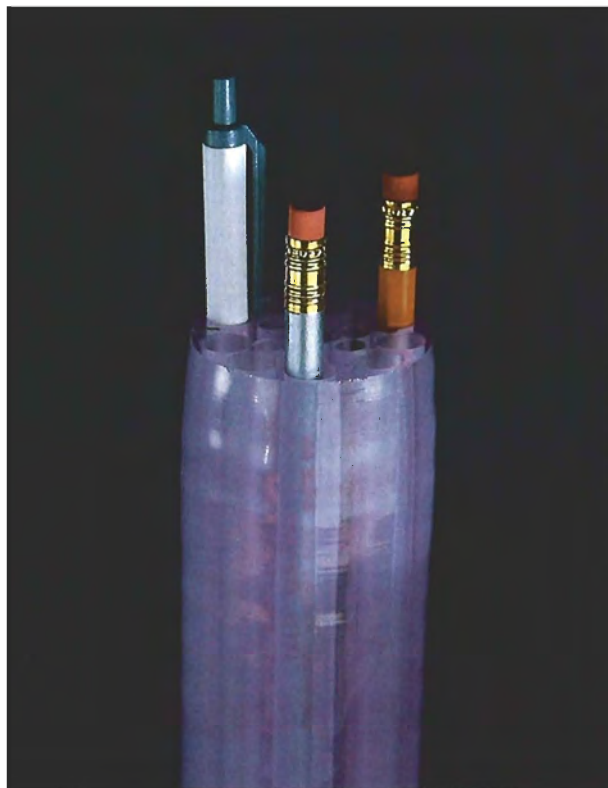
Figure 18. Standing approximately 6.25-in. (15.9 cm) tall, this cored crystal section of colored YAG was marketed as a "pencil holder." Photo by Maha Smith.
