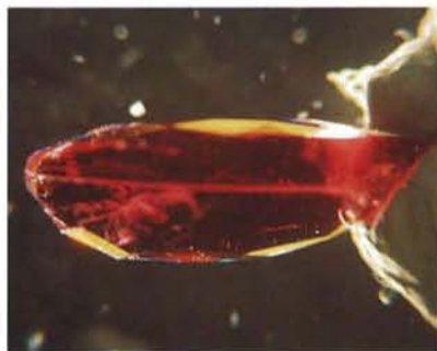
Figure 17. This profile view shows the separation plane of a ruby/ruby doublet. Immersion, magnified 17×.
