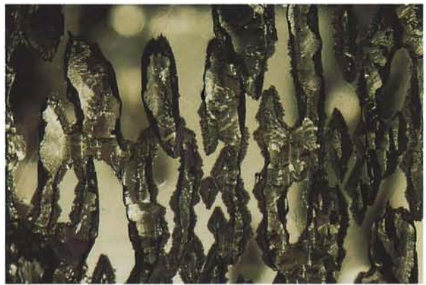
Figure 4. Deep surface etching is evident on the prism face of a 9.74 ct heliodor crystal from Tajikistan. Field of view, about 5.5 mm; photomicrograph by John I. Koivula.
