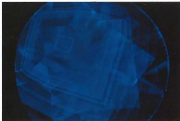
Figure 15. The square pattern revealed by cathodoluminescence means that the table facet of this diamond was oriented along a possible cube face in the original crystal. Photo by Junko Shida.
