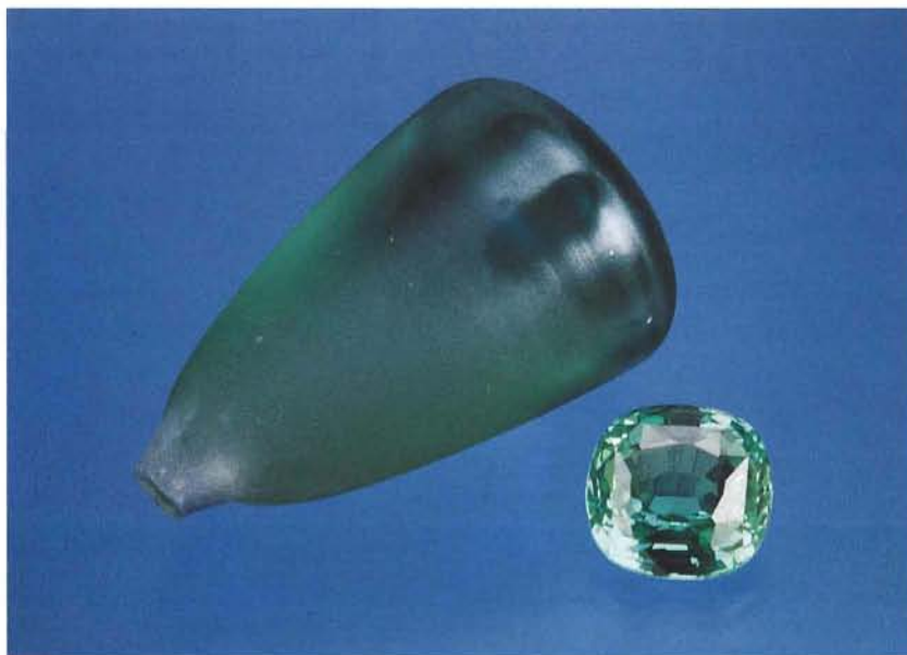
Figure 20. The origin of this 5.90 ct synthetic sapphire, shown here with a 116.71 ct boule of green synthetic sapphire, was determined on the basis of its absorption spectrum and inclusions.
