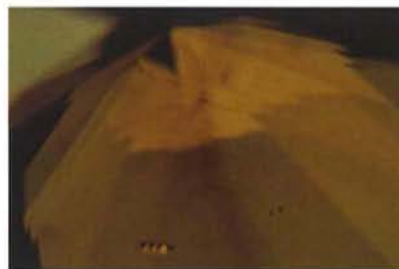
Figure 3. From another angle, the graining seen in this synthetic diamond shows a pattern closer to what has been reported previously in Russian synthetic diamonds, and unlike anything one would see in a natural diamond. Magnified 30 \times .
