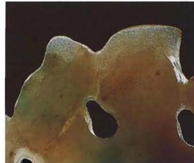
Figure 11. Magnification revealed not only that a piece at the top of the jadeite carving shown in figure 10 had been glued back on, but also that an adjacent area had been "reconstructed" with a polymer-like substance. Magnified 10×.
