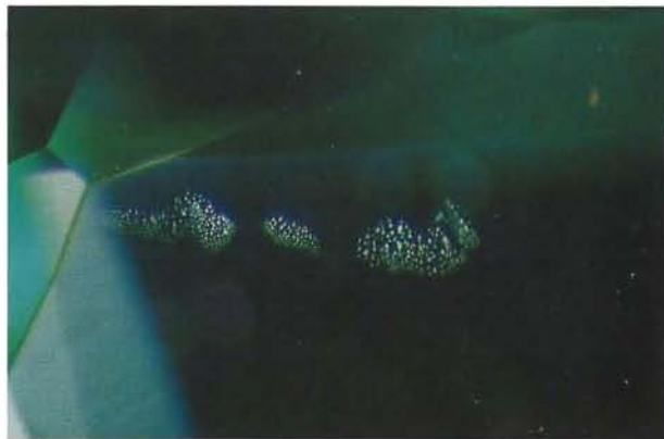
Figure 5. Only one fingerprint-like pattern was observed in any of the eight samples of Russian synthetic emeralds. Photomicrograph by John I. Koivula, magnified 35 \times .
