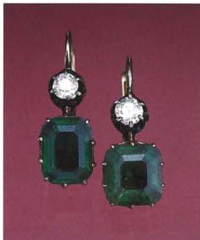
Figure 5. The green emerald cut in the earring on the right was identified as a natural emerald, while the emerald cut on the left was found to be a triplet consisting of a rock crystal quartz crown joined by green cement to a pavilion fashioned from an undetermined material.
