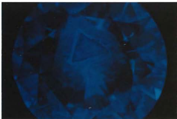
Figure 14. Cathodoluminescence reveals that the table facet of this diamond was oriented almost parallel to an octahedral face on the original crystal. Photo by Junko Shida.
