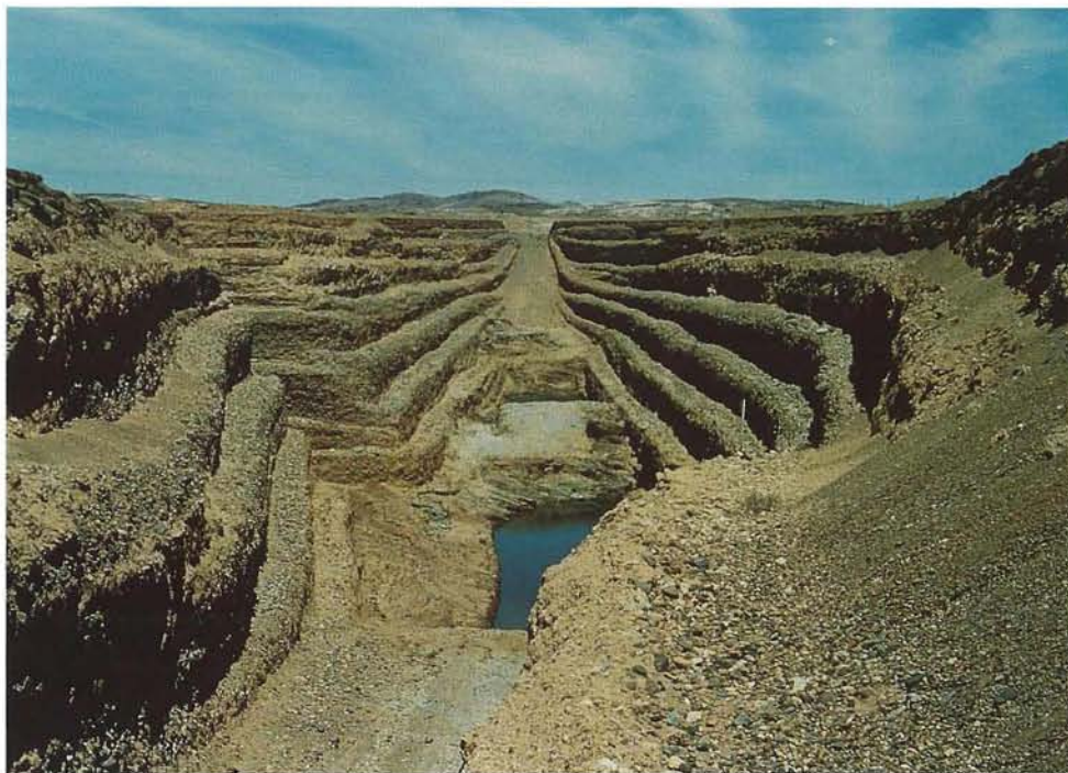
Figure 13. At the alluvial terrace deposit known as Auchas, on the Namibian bank of the lower Orange River, this prospecting trench has been cut through the deep overburden to reach the diamond-bearing gravels. Photo by Manfred Marx.
