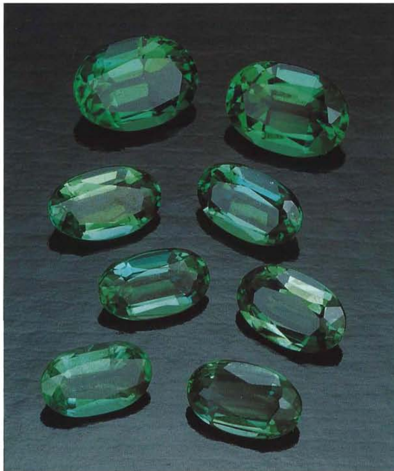
Figure 1. The eight Russian hydrothermal synthetic emeralds examined for this report, all oval mixed cuts, ranged from 0.17 to 0.41 ct. Photo by Maha DeMaggio.
