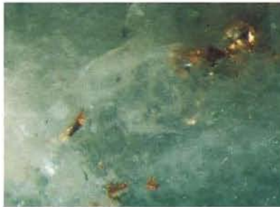
Figure 8. These metallic brownish orange flakes were seen in a bead of jadeite jade that was reportedly from Central America. They proved to be copper. Magnified 15 \times .
