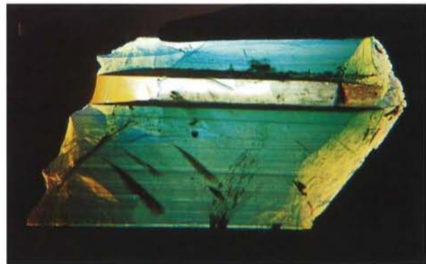
Figure 3. In this sample of the new type of Russian hydrothermal emerald, we can see a colorless seed plate and growth zoning parallel to the seed/synthetic emerald boundary at a 45 ^\circ angle to the c-axis. Crossed polarizers, immersion, magnified 16 \times .
