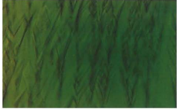
Figure 2. Also in the earlier production of Russian hydrothermal emerald, boundaries between subindividuals appear as an angular growth pattern. Immersion, magnified 45 \times .
