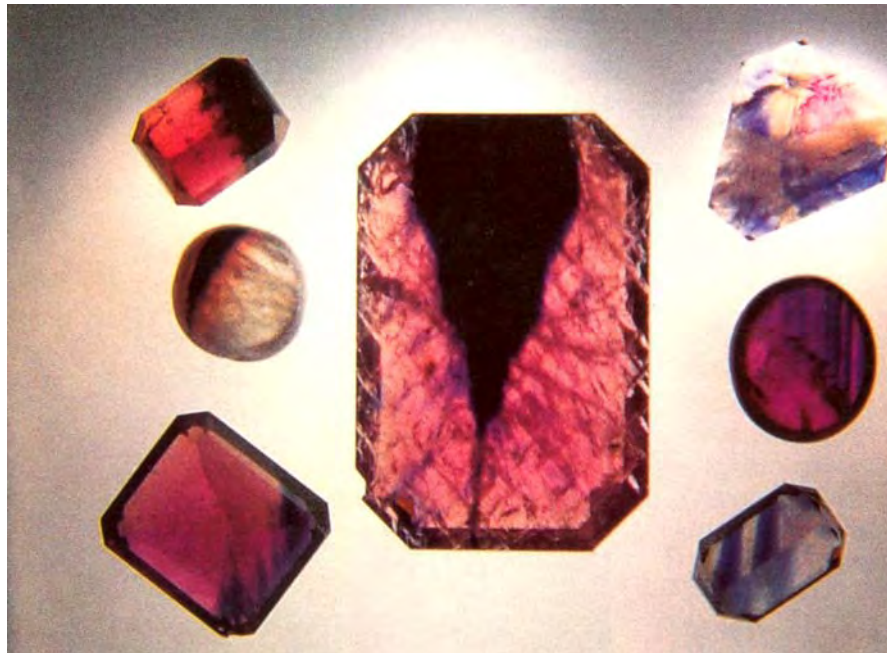
Figure 13. Distinct color zoning was present in most of the sample rubies and sapphires from Nepal. Colorless, red/pink, and dark violetish blue zones filled large sections of the stones, traversed them in bands, or appeared as large wedge-like forms. Such color-zoning characteristics gave many of the gemstones a bicolored appearance.
