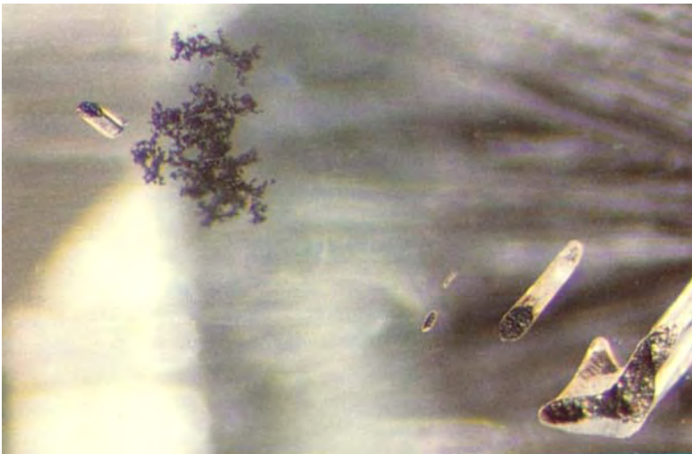
Figure 9. An unusual dendritic inclusion accompanies the elongate inclusions in this 1.25 ct Sumitomo synthetic diamond crystal (reference no. 21705). Photomicrograph by John I. Koivula; transmitted light, magnified 20 \times .
