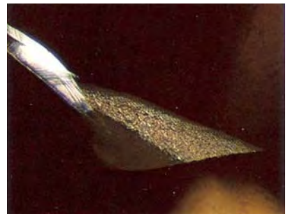
Figure 2. An etched feather can be seen in the pavilion of the Kelsey Lake diamond shown in figure 1. Magnified 57x.
