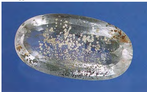
Figure 15. Aventurescence in this 70.48 ct rock crystal quartz is caused by light reflecting off a multitude of pyrite inclusions. Photo by Maha DeMaggio.
