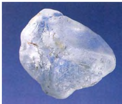
Figure 14. Trigons were engraved on this 17.56 ct colorless topaz rough to make it look like a diamond.
