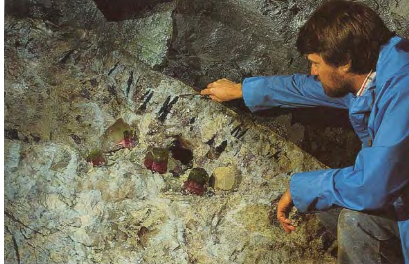
Figure 2. This pegmatite pocket from California's Himalaya mine yielded thousands of carats of fine tourmaline. Unfortunately, the discovery of such pockets typically requires hundreds of meters of tunneling and a great deal of luck. Rapid improvements in geophysical prospecting techniques offer the hope that this situation will change in the near future. Photo © Harold & Erica Van Pelt.
