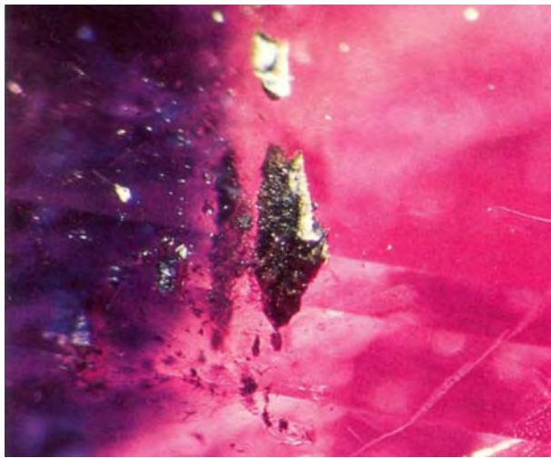
Figure 22. A series of unusual granular masses were identified as uvite tourmaline, which has not been documented as an inclusion in rubies from any other source. It thus provides a useful indication of Nepalese origin. Fiber-optic illumination, magnified 35x.
