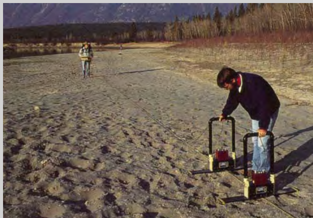
Figure C-3. The equipment required for georadar is very portable, and the procedure is not labor intensive. In this photo of a georadar field crew working in western Canada, the person in the foreground is setting the antennas, one for transmitting the radar pulse and the other for receiving the returned signal. The person in the background is carrying the instruments that control the signals and record them onto magnetic tape or disk. The wire along the ground connects the antennas to the recording instruments. Photo courtesy of D. G. Smith.
