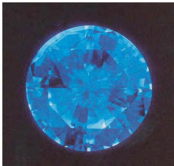
Figure 8. Like fluorescence, cathodoluminescence in near-colorless synthetic diamonds is also typically uneven and very different from the patterns seen in natural diamonds. A faint cross shape is visible in this 0.61 ct near-colorless De Beers synthetic diamond (reference no. 30100). Photo by Shane Elen.
