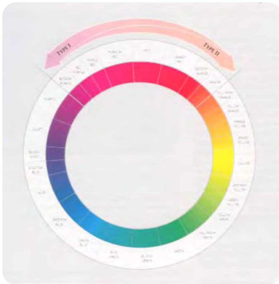
Figure 5. This diagram illustrates the relatively wide range of hues in diamonds (indicated by the arrows) that GIA GTL associates with the term pink.
