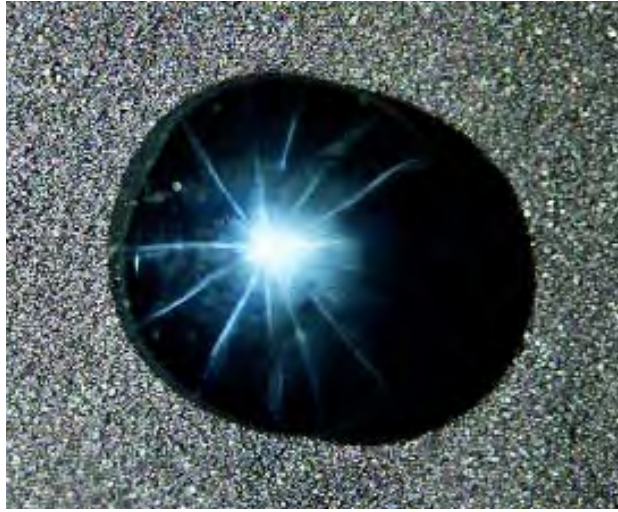
Figure 33. This 45.45 ct rutile with man-made asterism shows an 11-rayed asymmetric star with incomplete arms. Some of the arms also are split at the outer region of the cabochon. The star is sharp, but the stone appears fuzzy because the camera is focused below the cabochon's curved upper surface. Photo by M. Glas.
