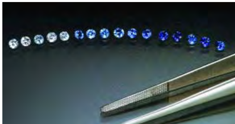
Figure 8. Benitoite melee is now being faceted in full round brilliants with a consistent set of proportions. A range of colors is available, as shown here (0.07 ct each). Courtesy of Benitoite Mining Inc. and Iteco Inc.; photo by Robert Weldon.
