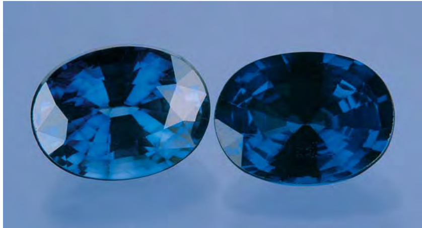
Figure 12. These two sapphires (2.74 and 2.23 ct) were submitted to the laboratory together. The lighter one (left) showed evidence of standard diffusion treatment with titanium. The darker stone was colored by a very shallow surface layer that contained cobalt.
