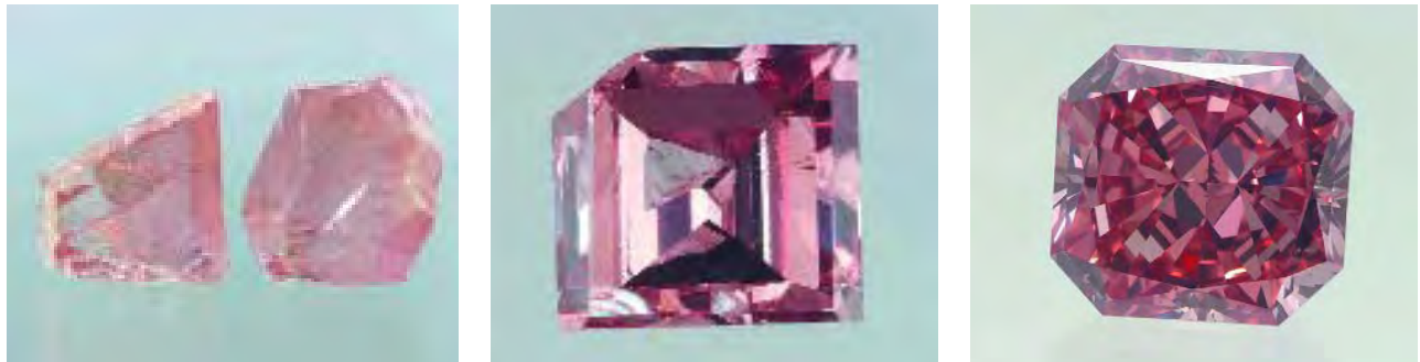
Figure 21. When pink diamonds are manufactured, the potential difference in color appearance between the rough and the faceted gem can be dramatic. This series show the original cleaved rough (left), the gem being cut from this rough at an interim stage in the faceting process (17.39 ct; middle), and the final 12.74 ct Fancy Vivid orangy pink diamond (right). Courtesy of Jacques Mouw; photos by Elizabeth Schrader.
