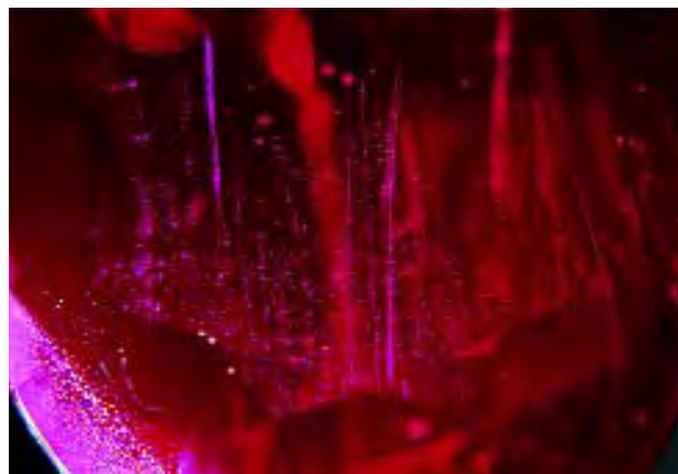
Figure 32. Very fine, parallel to subparallel stringers of pinpoints also were visible in the unusual flux-grown synthetic rubies. Photomicrograph by Christopher P. Smith; magnified 18 \times .
