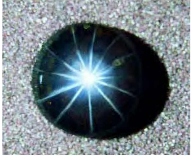
Figure 34. This yellowish brown, slightly translucent tourmaline (13.14 ct) with man-made asterism displays a 12-rayed, asymmetric star with additional "satellite" lines in the center of the sample. As in figure 33, the stone appears fuzzy (and the star sharp) because the camera is focused below the upper surface of the cabochon. Photo by M. Glas.
