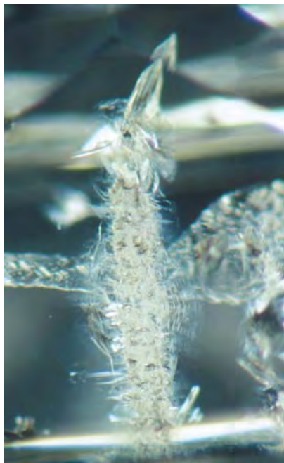
Figure 7. Internal laser drilling can create a series of small step-like feathers that connect an inclusion to the surface of the diamond, often leaving behind a white area with a sugary texture in the center of the feathers. Magnified 37 \times .
