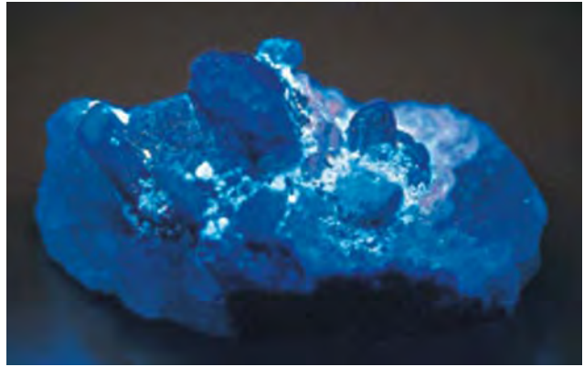
Figure 19. This cleverly assembled imitation of a tanzanite mineral specimen ( 5.5 \times 3.0 \times 1.0 cm) contains pieces of grayish purple tanzanite, light green diopside, and smoky quartz glued onto a matrix of calcite and graphite (left). With exposure to long-wave UV radiation (right), the glue mixture fluoresced bright white (the orangy pink areas are calcite). Photos by Maha Tannous.
