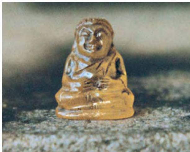
Figure 15. Buddha statues such as this one (2.5 cm tall) are being sold as amber carvings in Thailand. However, they are manufactured from cubic zirconia. Photo by Anne-Claude Couturier.
