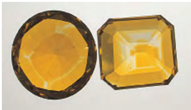
Figure 5. Immersion in water reveals the different color zoning patterns in these two yellow synthetic diamonds (0.60 and 0.49 ct; viewed table-down). These patterns depend on several factors: the shape and relative sizes of the faces on the original crystal, the area of the original crystal contained within the faceted sample, the orientation of the crystal relative to the facet arrangement, and the relative distribution of nitrogen between growth sectors. Photomicrograph by J. E. Shigley.
