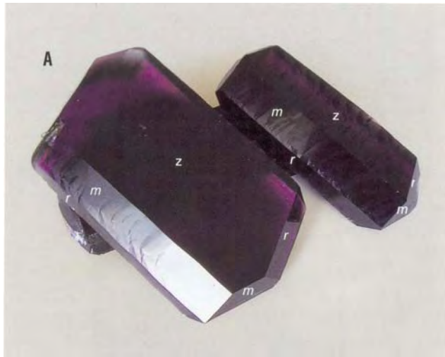
Figure 3. The synthetic amethyst crystals in image A show the typical morphology resulting from growth in alkaline K_2CO_3 solutions on seeds cut parallel to z; the largest crystal is 23 cm long. Image B shows polished slices that were cut from such crystals (2 mm thick, sliced parallel to a). Note the colorless seed plate along the center of each slice. The crystals are formed mainly by z growth sectors, while r sectors occupy small portions. Faceted synthetic amethysts prepared from such crystals consist almost entirely of the z sector. However, Dauphiné twinning may augment the r sectors in such crystals (see bottom slice), so that faceted material may contain both z and r sectors. Photos by V. S. Balitsky (image A) and Maha Tannous (image B).
