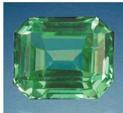
Figure 14. This 8.85 ct light yellowish green emerald cut submitted for an emerald report was identified as a synthetic sapphire. Its unusual color is attributed to a combination of cobalt and vanadium.
