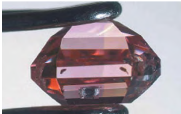
Figure 32. The color zoning seen in these pink synthetic diamonds consisted of distinct areas of purplish pink and orangy pink with sharp, well-defined borders. Photomicrograph by James Shigley; magnified 15x.
