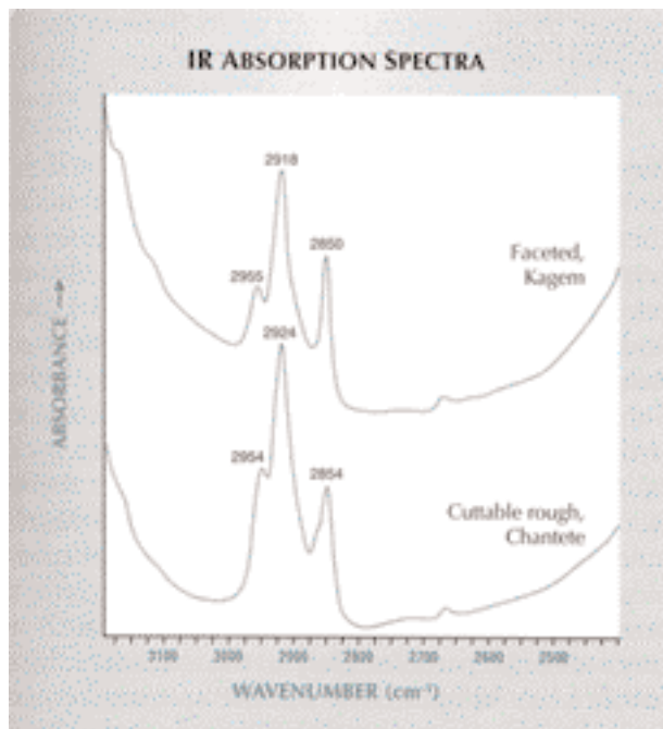
Figure 41. Peaks in the 3100–2800 \text{cm}^{-1} range were seen in the FTIR spectra of both faceted and cuttable rough specimens of Kafubu emerald, indicating the presence of oil. No artificial resin was found in the stones that were tested. Spectra have been offset vertically for clarity.
