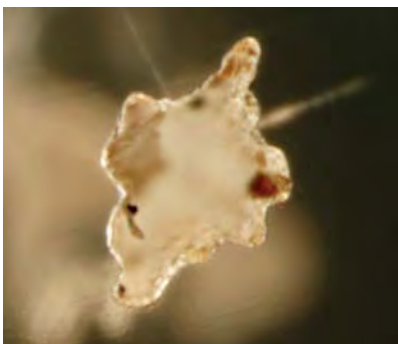
Figure 18. Where the drill holes reach the surface of the diamond, they show an unusual outline, again unlike any previously encountered in the lab. Magnified 105x.
