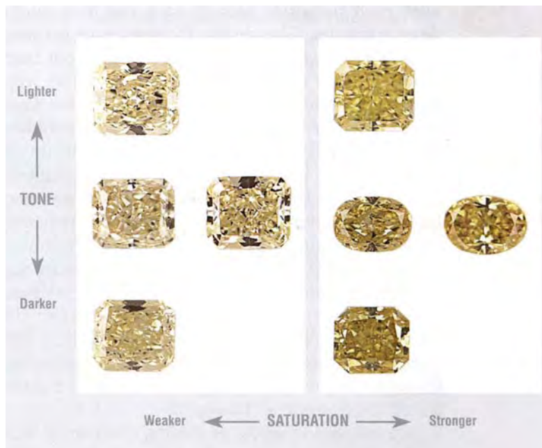
Figure 24. If a diamond is near a grade boundary, darker tone can be confused with increasing saturation if known references are not used. Here, two examples illustrate this situation. On the far left are three diamonds near the Y-Z/Fancy Light yellow saturation boundary; the diamonds are of similar saturation and differ only in tone. Comparison to the Fancy Light yellow reference diamond to their right establishes their grade on the D-to-Z scale. On the right, a similar situation is seen with three diamonds near the Fancy Intense/Fancy Vivid boundary; their Fancy Intense grade is clear when they are compared to the Fancy Vivid yellow reference diamond to their right. These tonal differences can be misinterpreted by an inexperienced observer. Photos by Elizabeth Schrader.
