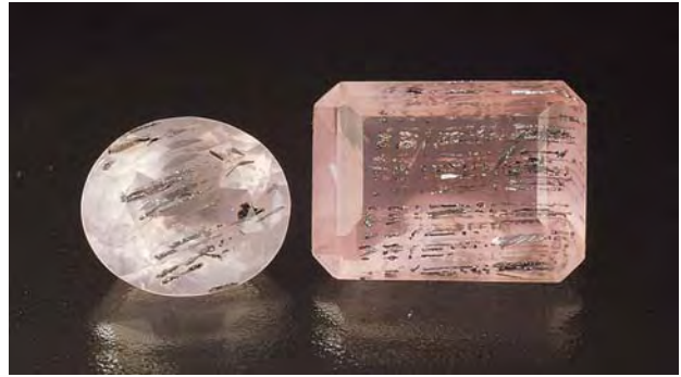
Figure 12. These faceted samples of rose quartz (5.74 and 12.55 ct) from the Itongafeno pegmatite in central Madagascar contain conspicuous inclusions of bismuthinite. Photo by J. Hyrsl.
