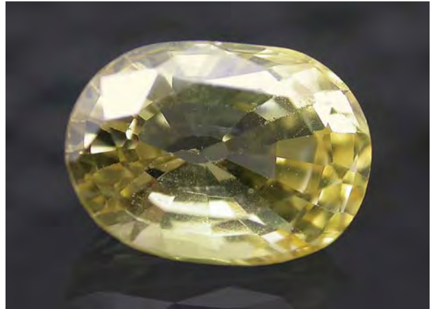
Figure 14. The slightly brownish yellow body color of this 4.30 ct hydrothermal synthetic sapphire is characteristic of those encountered at the Gem Testing Laboratory in Jaipur, India. Photo by G. Choudhary.
