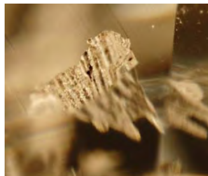
Figure 19. Dark, rounded grooves along the length of this cavity in the 8.38 ct diamond are further indications of laser drilling. Magnified 45x.
