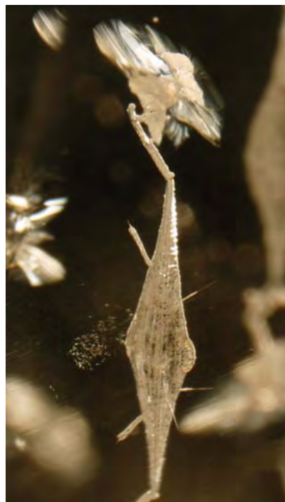
Figure 17. This large cavity in an 8.38 ct diamond does not resemble any natural etch channels or laser drill holes seen previously in the laboratory. Magnified 35x.
