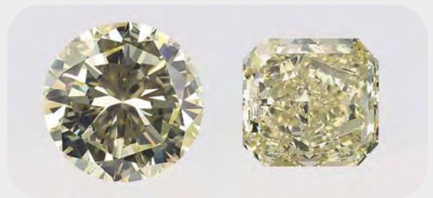
Figure A-2. Some of the most striking differences are seen when a light yellow round brilliant is recut into a shape and cutting style, such as the radiant, that can accentuate the color appearance. For example, the 6+ ct round brilliant diamond on the left was graded in the W-X range of the D-to-Z scale. When recut as a 4.61 ct radiant (right), it was graded Fancy yellow. Courtesy of the Scarselli family; composite photo by Elizabeth Schrader.
