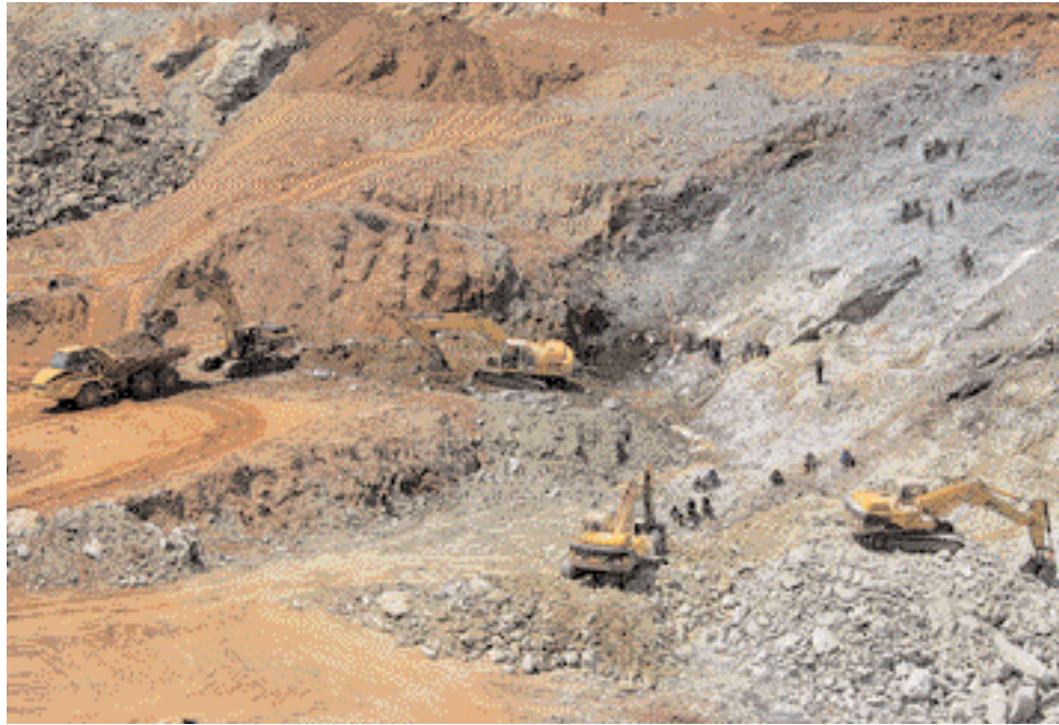
Figure 5. The Grizzly mine employs large earth-moving equipment in a highly mechanized operation. The excavators used in the Kafubu emerald mines typically weigh 25–30 tons and have a bucket capacity of approximately 1.6 m 3 . Photo by B. M. Laurs.
