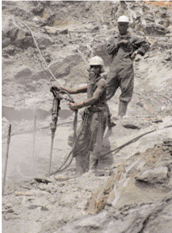
Figure 6. At the Grizzly mine, workers drill holes that will be filled with explosives to open up the area adjacent to an emerald-bearing zone. Photo by B. M. Laurs.
