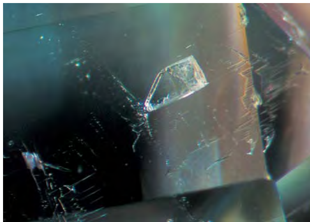
Figure 15. This inclusion in a Mt. Mica tourmaline was identified as feldspar by Raman analysis. Fluid inclusions also are visible in the immediate vicinity. Photomicrograph by John I. Koivula; magnified 20x.
