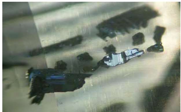
Figure 13. The bismuthinite inclusions in the rose quartz from Madagascar appeared metallic gray to black, and showed a variety of irregular forms. A network of needle-like inclusions, possibly rutile, was responsible for the asterism in this rose quartz. Photomicrograph by J. Hyrsl; the field of view is approximately 3 mm.
