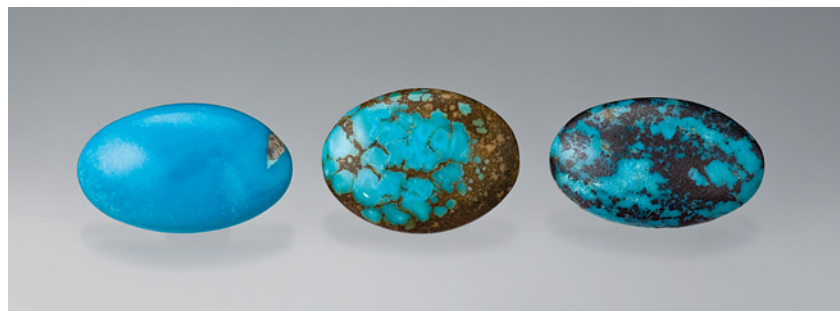
Figure 13. These three cabochons (5.93–8.08 ct) were treated by the Eljen process and studied for this report.
