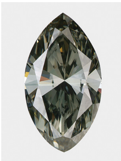
Figure 5. This highly unusual Fancy Dark gray-green diamond ( 16.54 \times 9.13 \times 5.87 mm) proved to be type IIb.
