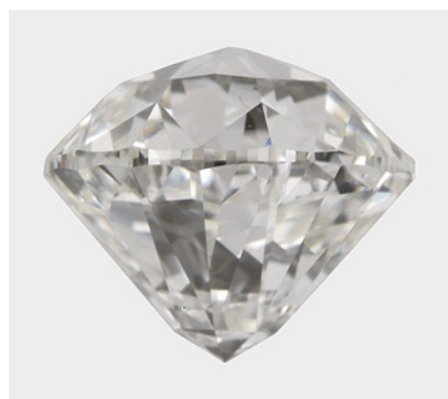
Figure 7. This side view of the 2.08 ct round-cut Antwerp Twins diamond in figure 6 shows the unusual “dome” faceting of the crown and pavilion.
