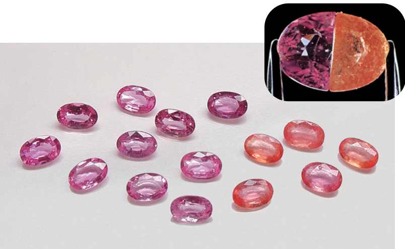
Figure 13. In 2002, the industry learned that beryllium diffusion was being used to significantly alter the color of corundum, changing pink stones (such as those on the left of this photo by Sriurai Scarratt) to pink-orange after treatment (right). This was dramatically illustrated by Shane McClure's inset photo of a 0.51 ct pink sapphire that had been cut in half, with the portion on the right undergoing Be diffusion.
