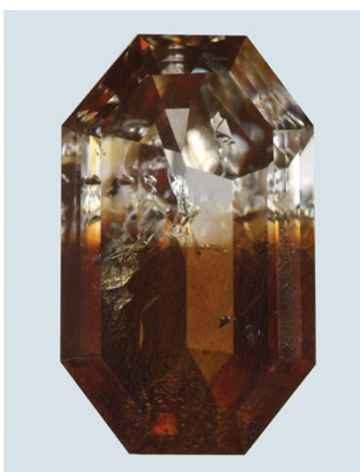
Figure 1. This unusual diamond (1.79 ct) proved to be a mixed-type IaA/Ib, with the two types corresponding to the near-colorless and Fancy Dark orangy brown regions, respectively.
