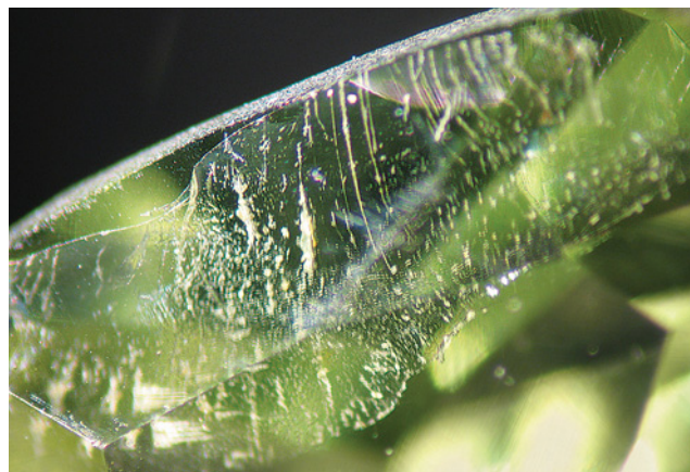
Figure 4. Sardinian peridot commonly contains partially healed fractures (left, magnified 30 \times ). Decrepitation halo cleavages were present in some of the samples (right, magnified 45 \times ). Photomicrographs by I. Adamo.
