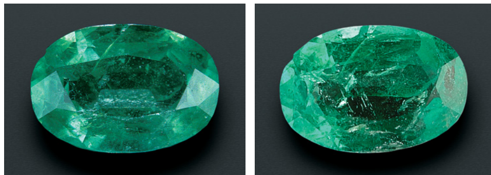
Figure 14. Mary Johnson's 2007 article on emerald fillers investigated their durability over time and under common conditions of wear and cleaning. The fissures in this 0.74 ct emerald filled with Araldite 6010 (left) partially emptied out after 30 minutes of ultrasonic cleaning (right).
