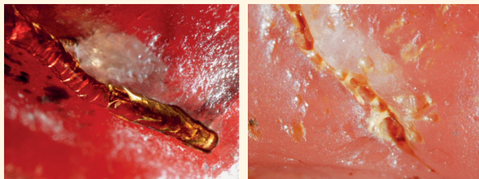
Figure 12. Channels on these andesines are filled with a transparent yellow-brown glassy material (left, known-treated stone, image width 2.9 mm) or an opaque yellow substance partially bridging the gap in the specimen (right, from Zha Lin, image width 1.75 mm). Photomicrographs by S. F. McClure.
