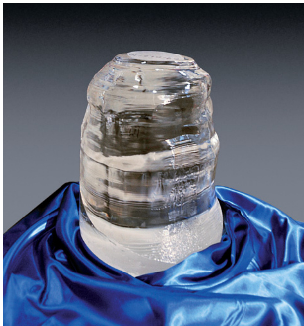
Rubicon's first synthetic sapphire grown by the Kyropoulos method at their new plant in Batavia, Illinois, measured ~30 cm in diameter. Courtesy of Business Wire.
