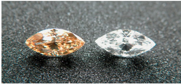
Significant color changes are produced by HPHT treatment of natural type IIa diamond. The brown diamond is 0.82 ct and the HPHT-treated colorless stone is 0.84 ct. Courtesy of the DTC Research Centre.
