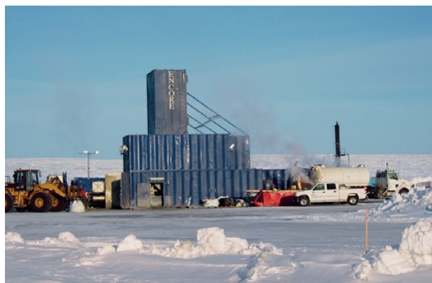
Shown here is a kimberlite bulk sampling operation (large diameter drilling) at the DO-27 kimberlite, Northwest Territories, Canada, in March 2006. Photo by H. G. Coopersmith.
