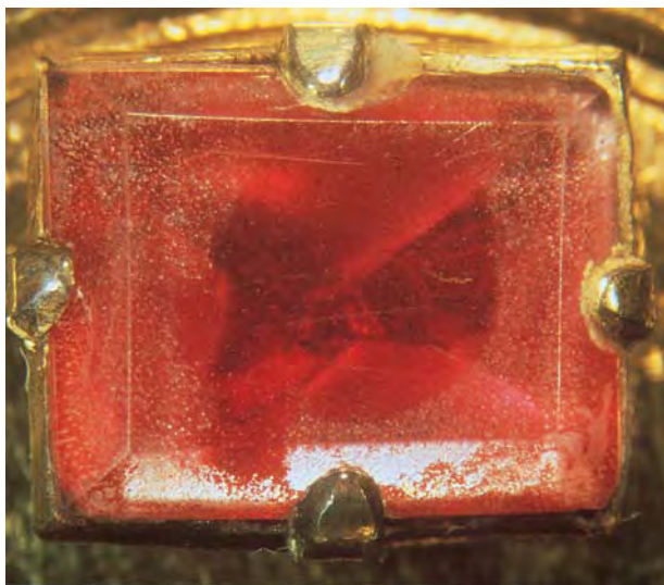
Figure 4. Four of the stones tested were found (by microscopy and Raman analysis) to be doublets with quartz tops and a layer of red cement. This stone, in the Reliquary cross, measures 10.7 \times 8.6 mm.
