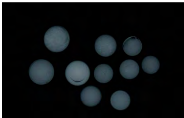
Figure 9. In this X-radiograph, the pearls cultured on dolomite beads have a very different appearance from the Tahitian black cultured pearl placed in the center as a reference.
