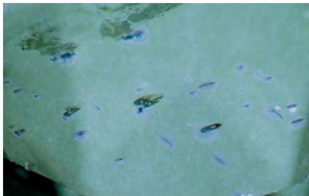
Figure 21. Blue color concentrations can be seen around several minute fractures on the table of this surface-treated topaz. Photomicrograph by Shane F. McClure; magnified 23 \times .
