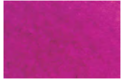
Figure 13. Closer examination of the cabochon shown in figure 12 revealed the characteristic appearance of a dyed aggregate material, in this case quartzite. Magnified 30×.
