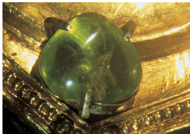
Figure 8. Raman analysis identified this 10.7 \times 9.3 mm stone in the Dorothy monstrance as peridot.
