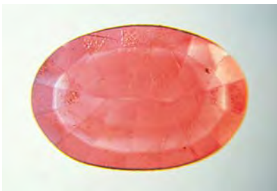
Figure 2. When immersed in methylene iodide and placed over diffused transmitted light, this 0.69 ct oval mixed-cut corundum showed both the color concentrations on facet junctions and the spots devoid of color that indicate that it was colored by diffusion treatment.
