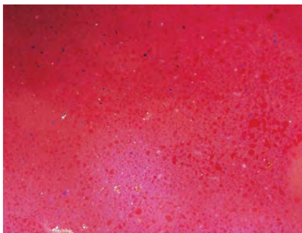
Figure 5. Red pigment is seen here mixed in the cement of the doublet in figure 4. Magnified 60\times
