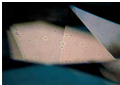
Figure 4. The spotty surface coating on the diamond shown in figure 3 was revealed with magnification (here, 63 \times ) and a diffuse light source.
