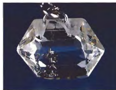
Figure 2. This diamond, which measures 11.65 \times 9.75 \times 5.60 mm and weighs about 6.5 ct, was cut along the original crystal shape and drilled at an angle from each end for mounting.
