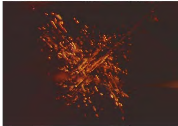
Figure 7. Acicular inclusions were the only internal feature seen in the Mozambique garnets shown in figure 6. Photomicrograph by John I. Koivula, magnified 30x.
