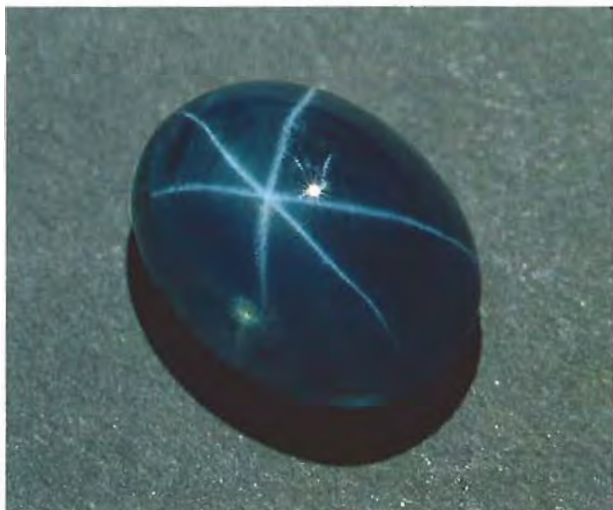
Figure 19. The star in this 3.73 ct (9.18 × 6.82 × 5.39 mm) sapphire was produced by a surface diffusion treatment. Photo by Maha DeMaggio.
