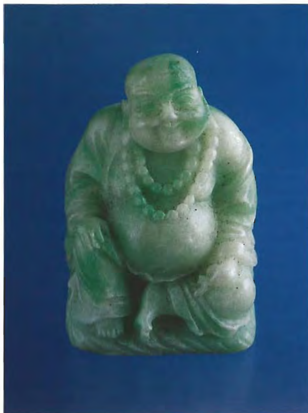
Figure 20. This 239.37 ct imitation jadeite statuette (47.35 × 32.90 × 32.75 mm) is composed of finely ground calcite in a groundmass of alkyd resin polymer (plastic). The green areas were probably produced by selective dyeing. Photo by Maha DeMaggio.
