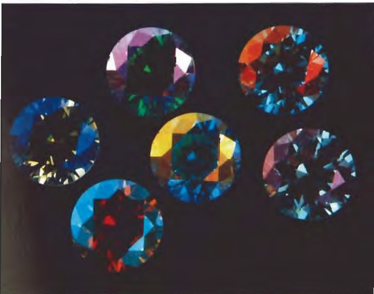
Figure 23. These six 4-mm-diameter samples (about 0.46 ct each) of a cubic zirconia marketed as "Tavalite" owe their colors to thin optical coatings. Photo by Maha DeMaggio.
