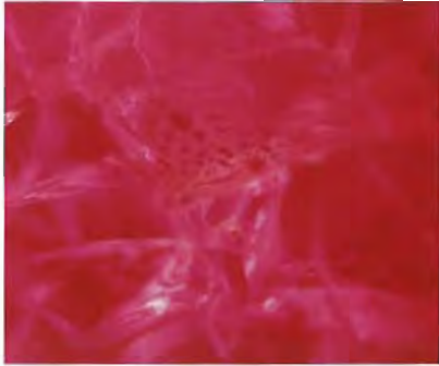
Figure 14. Some of the fractures induced in the synthetic ruby cabochons shown in figure 12 had the appearance of natural fingerprint inclusions. Magnified 40x.
