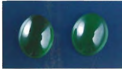
Figure 5. These natural-color jadeite cabochons appeared red when examined with a Chelsea color filter, which could lead a gemologist to falsely suspect that they were dyed.
