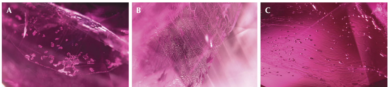
Figure 21. A: This healed fracture has irregular droplets of flux that were trapped during healing. They stand out due to their high relief and more translucent appearance; field of view 2.88 mm. B: Connecting networks of trapped flux in a healed fracture; field of view 2.80 mm. C: Not all fractures were able to heal to the same degree. Swirling droplets of trapped flux and air reveal that a large portion of this fracture is actually filled with solidified flux rather than healed corundum; field of view 1.20 mm. Photomicrographs by C. Khowpong (A and B) and S. Wongchacree (C).
