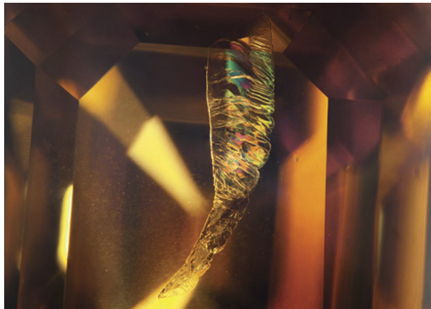
Figure 6. A subsurface feather in diamond resembling an insect wing, with visible iridescence caused by thin-film interference. Photomicrograph by Matthew Hardman; field of view 2.90 mm.
