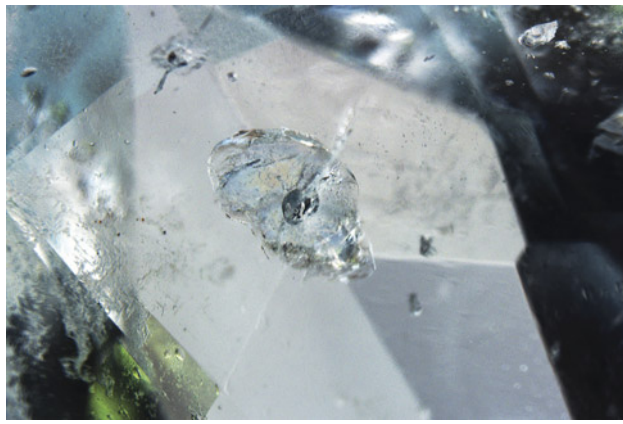
Figure 3. Disk-shaped fissures in the aquamarine were caused by solid inclusions in the middle with tubular fissures extending inward. Photomicrograph by Yubing Chen; field of view 1.50 mm.
