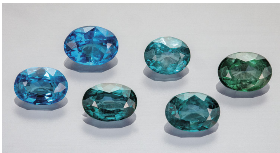
Figure 1. Suite of faceted nickel-diffused spinel (0.67–1.01 ct) showing a range of color from blue to bluish green. Photo by Aaron Palke and Diego Sanchez.
