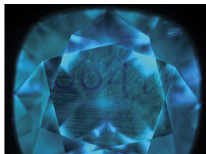
Figure 12. Left: The DiamondView image of the 1.93 ct CVD laboratory-grown diamond shows numbers on the table facet. Right: The 0.60 ct CVD laboratory-grown diamond shows a logo mark on the star facet.
