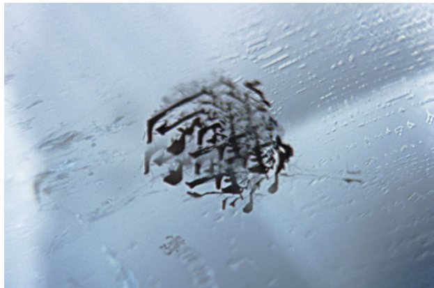
Figure 1. Hematite inclusions extend from the center of an aquamarine sample from Xinjiang, China. Photomicrograph by Yubing Chen; field of view 3.64 mm.
