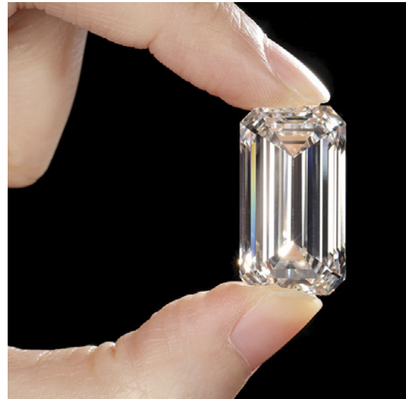
Figure 8. This 34.59 ct CVD-grown diamond ( 24.94 \times 13.95 \times 9.39 mm), produced by Ethereal Green Diamond in India, is the largest GIA has tested.
