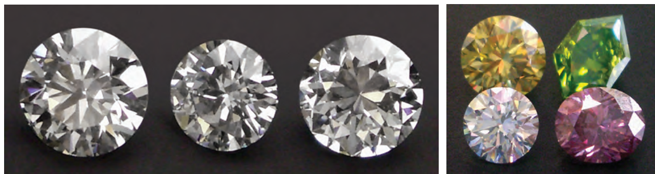
Figure 3. Untreated and treated natural diamonds were included in the study. On the left are three untreated samples provided by GIA: 0.64, 0.41, and 0.90 ct. On the right are four HPHT-treated natural diamonds from Suncrest Diamonds: a 0.43 ct colorless round, a 0.63 ct pink oval, a 0.66 ct green shield, and a 0.70 ct yellow round. Photos by K. Feral.
