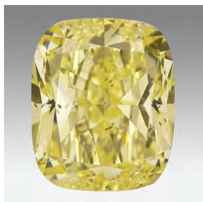
Figure 6. This 15.01 ct cushion-cut diamond ( 15.39 \times 12.84 \times 8.32 mm) was color graded as Fancy Intense yellow. Its color was found to have been treated from the original Fancy Light yellow.
