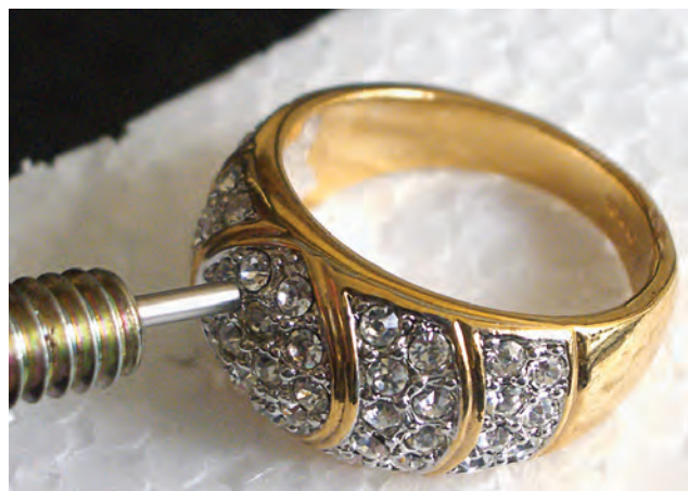
Figure 5. Pinpoint testing with flotation may be required to detect magnetic attraction in synthetic diamonds containing tiny metallic inclusions, such as the 1.07 ct yellow HPHT-grown sample on the left. This method can also be used to test individual small diamonds mounted in jewelry, as depicted on the right with a gold and diamond ring undergoing flotation testing. The raft material is Styrofoam. Photos by K. Feral.
