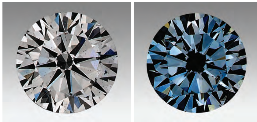
Figure 14. The [Si-V] - center was confirmed in these two HPHT-grown type IIb synthetic diamonds. The 0.51 ct round brilliant on the left was color graded as Fancy Light blue, and the 0.79 ct sample on the right had Fancy Deep blue color.
