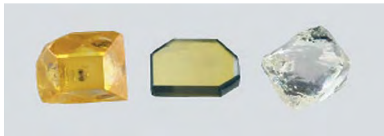
Figure 3. Due to the dramatic differences in their formation environments and growth mechanisms, CVD synthetic diamond crystals differ in appearance from natural diamonds, as well as from traditional HPHT-grown synthetic diamonds. HPHT synthetic diamonds (left) usually show well-developed \{111\} and \{100\} faces, and the flat surfaces have characteristic growth features. CVD-grown diamond crystals (center, no. 48922) usually have a tabular form, and \{111\} and \{110\} are poorly developed. Natural diamond crystals (right) may occur in any of several shapes that are very different from those of either CVD or HPHT synthetic diamonds. The octahedron is a very common form. Many natural diamonds display resorption features on their surfaces. Photo by Elizabeth Schrader.
