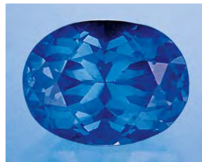
Figure 9. The high R.I. of this 5.42 ct violetish blue specimen of manufactured glass, very close to that of tanzanite, could lead to a misidentification.
