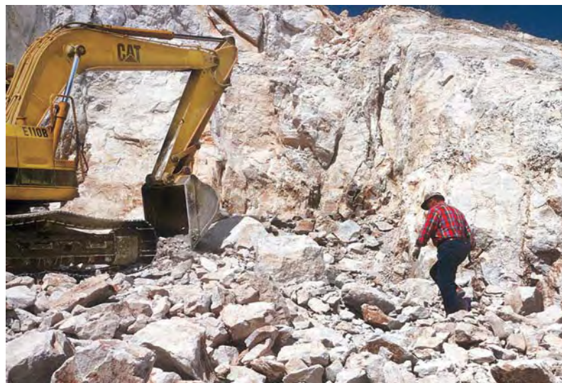
Figure 5. In this mineralized section of the Ruby Violet mine, a number of discontinuous, near-vertical fractures are exposed in the rhyolite host rock. The rhyolite is excavated with earth-moving equipment and hand tools to expose productive areas for red beryl that occur along these fractures. Mine owner Rex Harris is shown for scale; photo courtesy of William Rohtert, taken in 1995.
