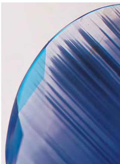
Figure 16. Often the color bands in the possibly new treated sapphires do not end at the light blue or near-colorless rim, but rather get abruptly lighter and appear curved. Immersion, magnified 10×.
