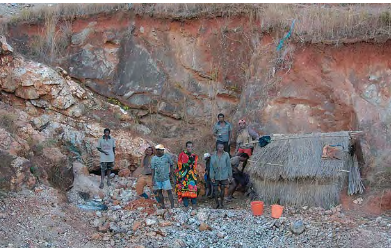
Figure 6. The Sakavalana pegmatite is visible in this open cut as the light-colored dike on the left. The miners are standing in front of a 13-m-deep shaft that produced multicolored tourmaline crystals. The entrance to a separate tunnel that leads upward to the pezzottaite workings is visible behind the man on the far left. The green color of portions of the pegmatite and mine dump is due to the presence of amazonite feldspar. Photo by Brendan Laurs.
