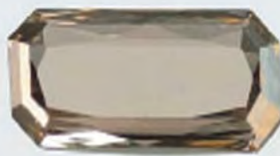
Figure A-2. As grown, this 0.45 ct CVD synthetic diamond (no. 57688) was light brown (left). After HPHT annealing, first at the graphite-stable region and then at the diamond-stable region, the sample showed virtually no change in color (right). Photos by Wuyi Wang.
