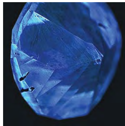
Figure 8. In this fluorescence image recorded with the DTC DiamondView, the cross-shaped zoning pattern typical of most synthetic diamonds is absent. The residue-filled surface cavities can be seen along the girdle on the left side of the diamond.
