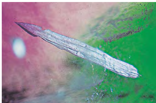
Figure 30. Raman analysis was used to identify the spear-shaped inclusions in the bi-colored fluorite as barite. Photomicrograph by John I. Koivula; magnified 10×.
