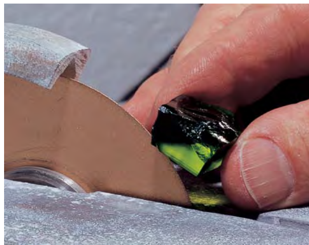
Figure 5. Sawing is one of the most important steps in gem cutting. The first series of cuts are made through cracks or veils (“fingerprints”) in the rough. Here, the preformer uses a high-speed, liquid-cooled saw with a 0.2 mm thick diamond blade on one of the peridots. Photo by Jeff Scovil.
