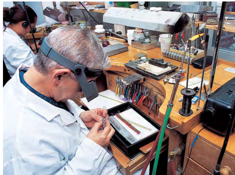
Figure 15. The jeweler hand-fabricates the hinges and connectors for the suite. For the bracelet, two platinum tubes were attached to the peridot settings and one to the settings for the baguette diamonds. Platinum hinge wires were inserted through the tubes to “join” the bracelet; the ends were then flanged. Photo by Robert Weldon.
