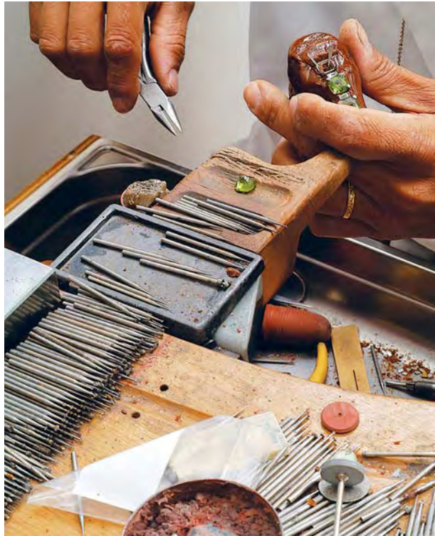
Figure 16. To set the peridots, a bracelet section comprising three main settings, with baguette diamonds separating the peridots, was put into a shellac stick on the end of a wooden handle. This stick allows the jeweler to firmly hold the section in one hand, while setting the gems using the appropriate tools. Photo by Robert Weldon.
