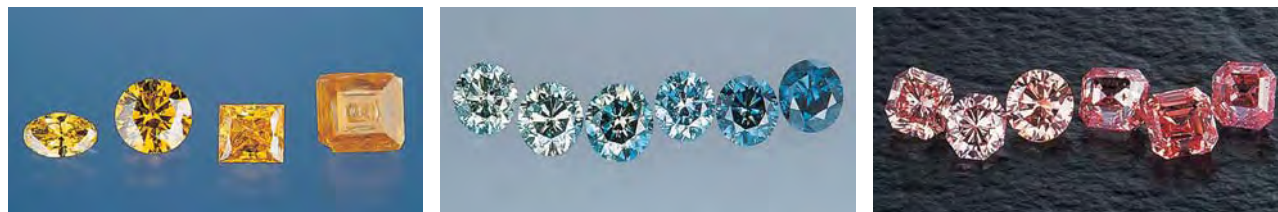
Figure 4. Synthetic diamonds currently sold for jewelry purposes display a range of as-grown and treated colors. The as-grown yellow crystal (2.43 ct) and three yellow faceted samples (0.28–0.84 ct) shown on the left represent the most common kind of synthetic diamond produced today. The colors of the green-to-blue faceted samples (0.20–0.40 ct) shown in the center also were produced during growth. In contrast, the pink-to-pinkish purple colors of the faceted samples (0.16–0.50 ct) shown on the right result from post-growth treatment processes. Photos by Maha Tannous.
