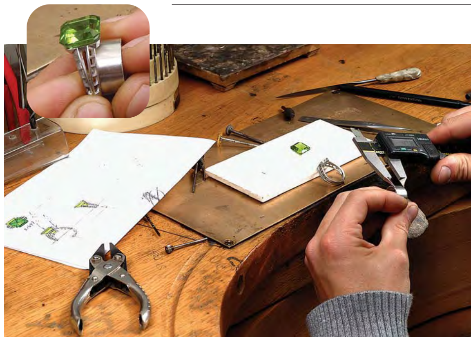
Figure 19. The main component of the ring was lost wax cast in platinum. The setting for the peridot (comprising the upper and lower galleries, and four prongs) was hand-fabricated from platinum sheet and wire. The upper inside-shank section was carefully fit to the ring (inset), before soldering and trimming. Photo by Robert Weldon.
