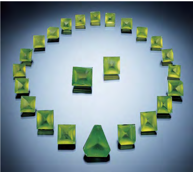
Figure 8. As the preforms were completed, they were laid out to check for consistency of color (hue, tone, and saturation) from one stone to the next and, for the necklace, to ensure the smooth graduation from large to small sizes. This photo shows the beginning stages of this process; as more preforms were completed they were added, and some (including a few of those shown here) were removed. Photo by Jeff Scovil.
