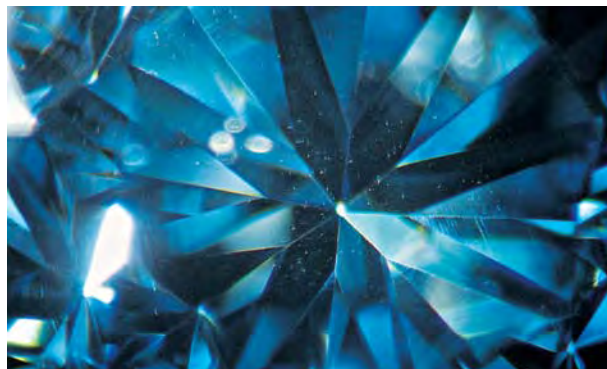
Figure 8. In some cases, synthetic diamonds display “clouds” of pinpoint inclusions of uncertain identity. Since some natural diamonds also exhibit similar cloud-like arrangements, these pinpoint inclusions do not provide a reliable means of separation. Photograph by Shane McClure; magnified 30×.
