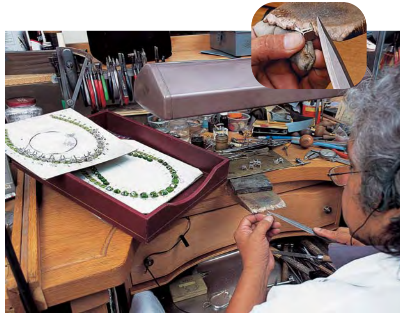
Figure 14. The setting (gallery and prongs) for each of the peridots was handmade to fit that stone. This photo shows the process underway. One tray holds the actual stones placed table-down over a color copy of the rendering; above this is a second tray with another copy of the rendering on which the settings have been placed in their proper position. The master jeweler then files and shapes each setting by hand to ensure the proper fit of the specific gem (inset). Photos by Robert Weldon.
