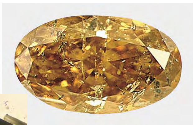
Figure 1. This 1.33 ct orangy yellow natural diamond displayed unusual Ni-related absorption features. The stone contains numerous hollow etch channels (see inset; magnified 25×), some of which appear dark in the photo of the diamond. Photos by F. Notari.
