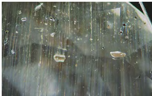
Figure 13. The jeremejevite also contained pale yellow crystals that could be feldspar or danburite. Photomicrograph by E. Fritsch; magnified 9 \times .
