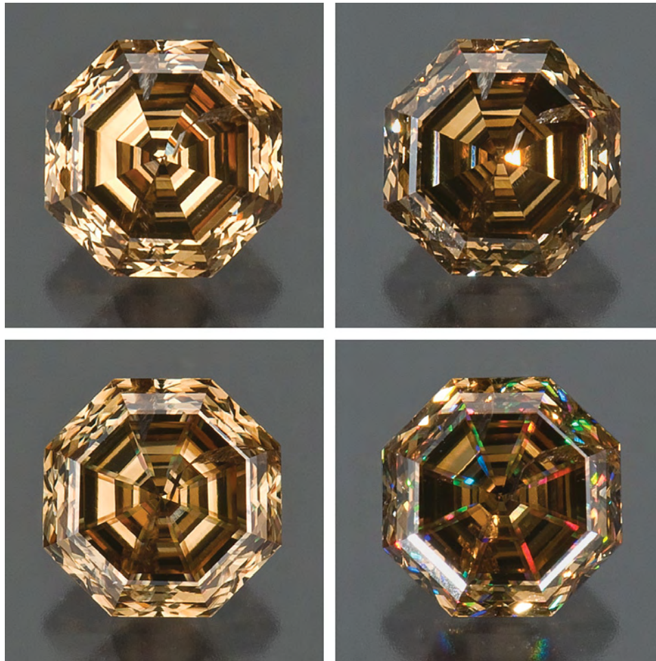
Figure 16. This octagonal step-cut fancy brown diamond (0.43 ct) is shown face-up in diffused light (top left) and spot lighting (top right) prior to plasma etching. In both instances, there is little fire. After processing with a modified pattern C adapted to this shape, the diamond looks much the same in diffused light (bottom left) but has a more dynamic face-up appearance and obvious fire in spot lighting (bottom right). Photos by Robert Weldon.
