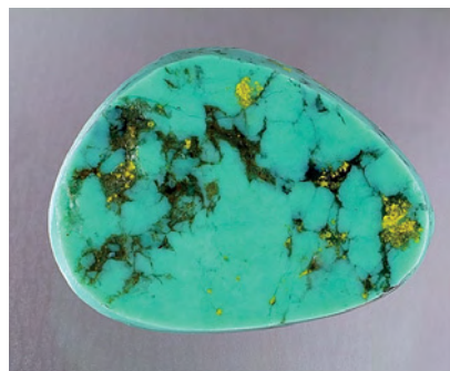
Figure 19. The GIA Laboratory recently examined turquoise beads and cabochons represented as coming from China, which have bright yellow inclusions of uranium-bearing francevillite. This specimen weighs 6.72 ct.
