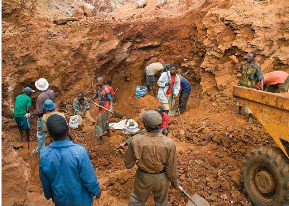
Figure 5. Shovels, pry bars, and picks are used to follow the gem-bearing veins. Photo by B. M. Laurs.
