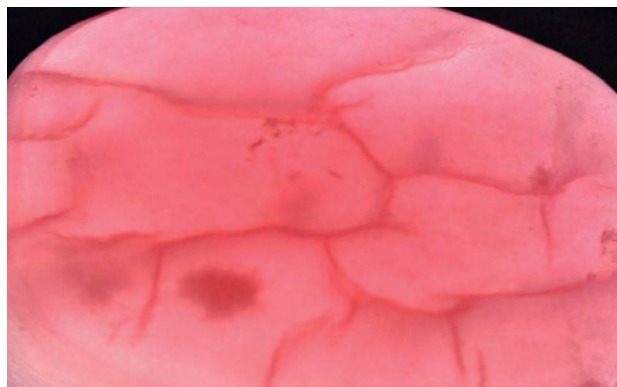
Figure 32. Surface-reaching cracks in the dyed alabaster displayed concentrations of red and pink. See also the curved color banding on the lower left. Photomicrograph by G. Choudhary; magnified 10 \times .
