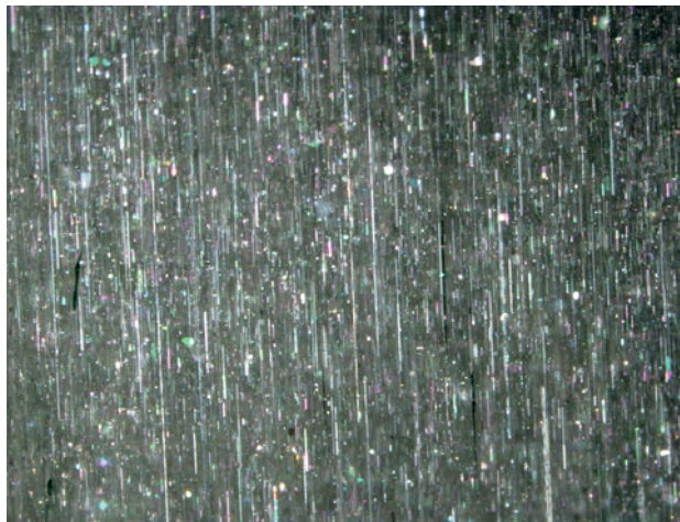
Figure 4. Abundant growth tubes and needles oriented parallel to the c -axis are responsible for the chatoyancy of the beryl. Raman analysis of the needles identified hematite (black) and siderite (white). Photomicrograph by W. L. Win; field of view 3.8 mm.
