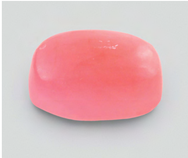
Figure 31. This 14.32 ct alabaster cabochon proved to be dyed; note its resemblance to opal or chalcedony. Also note the whitish chipped areas on the dome due to its very low hardness. Photo by G. Choudhary.
