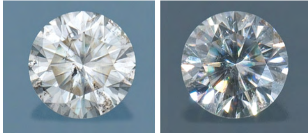
Figure 10. The grating pattern covers the entire pavilion of this 0.07 ct diamond. Modifying all the facet surfaces caused a reduction in overall brightness under diffused light (left). When examined with spot lighting (right), the diamond has an opalescent appearance and appears to be dirty or oily. Photos by Robert Weldon.
