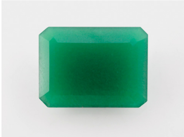
Figure 43. This 25.04 ct translucent green specimen, which proved to be glass, is unusual for its crystalline features. Photo by G. Choudhary.
