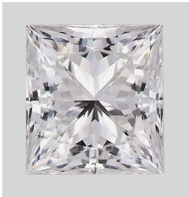
Figure 2. This near-colorless synthetic diamond (0.30 ct) illustrates the improvements in color and clarity seen in the later CVD-grown products offered by Apollo Diamond. Photo by Jian Xin Liao.
