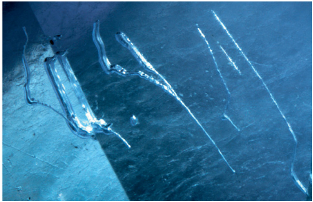
Figure 23. Significant amounts of neodymium and strontium were detected in this unusual 3.03 ct color-change synthetic apatite. Magnification (right) revealed features that indicated synthetic origin, such as these elongated gas bubbles. Left photo by Robert Weldon; right photomicrograph by J. I. Koivula, magnified 30 \times .
