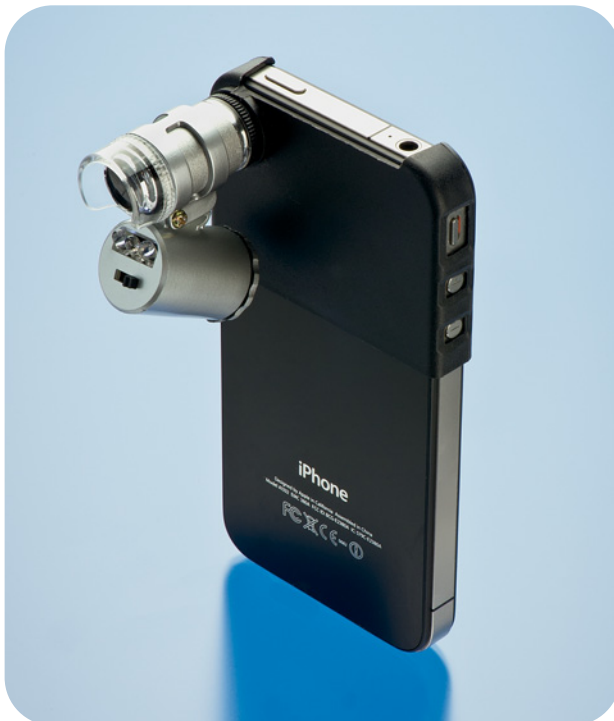
Figure 38. This inexpensive microscope accessory clips over a smartphone camera lens. Illumination is provided by LEDs. Photo by Robert Weldon.
