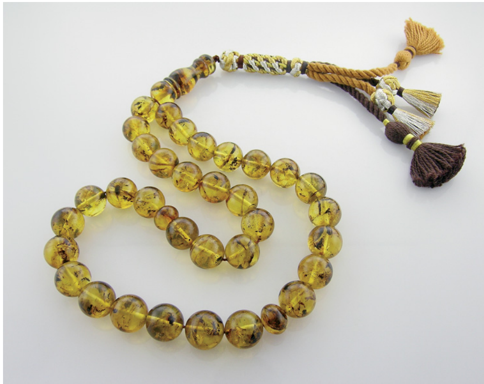
Figure 40. The beads in this rosary (~12 mm in diameter) proved to be copal filled and assembled with plastic to imitate amber. Photo by S. Singbamroong, © Dubai Central Laboratory.
