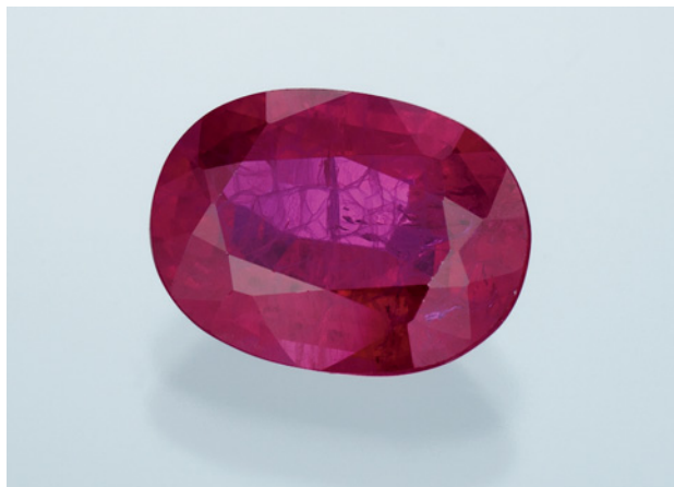
Figure 8. Containing numerous glass-filled surface-reaching cracks, this 3.50 ct flame-fusion synthetic ruby illustrates that synthetics can be treated, and that the presence of a treatment should not be construed as indicating natural origin. Photo by Robert Weldon.
