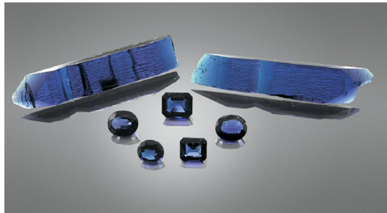
Figure 15. During the first decade of the 2000s, in addition to synthetic emeralds Malossi also produced hydrothermally grown synthetic aquamarines, such as the rough (14–16 g) and faceted (2.0–5.0 ct) material shown here. Photo by Alberto Malossi.
