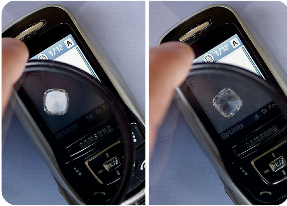
Figure 37. A simple polariscope is created when a polarizer is placed in front of the plane-polarized LCD screen. Here, a colorless topaz has been rotated on the cell phone screen under a camera polarizing filter. Photo B. Devouard.
