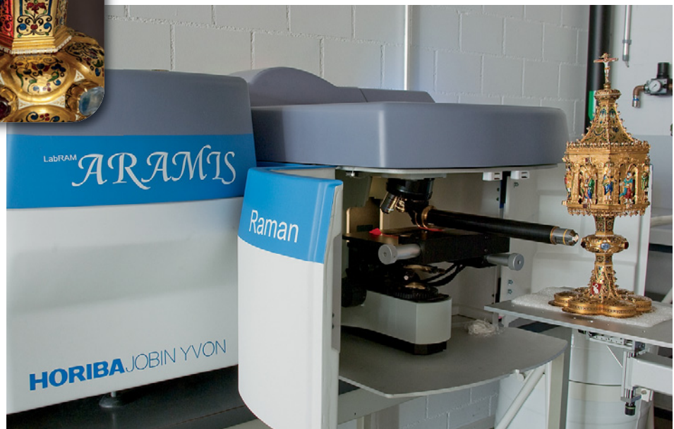
Figure 3. A Raman spectrometer with an L-shaped lens was used to take spectra on the mounted ciborium gems (inset), which were difficult to access with conventional equipment. All the stones were conclusively identified with this instrument. Photos by Michael Wörle.
