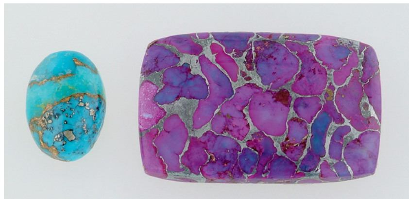
Figure 12. Artificial metallic veining is prominent in both of these composite turquoise cabochons (6.11 and 26.24 ct).
