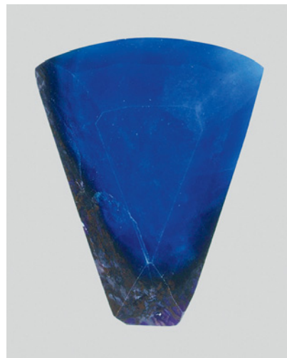
Figure 17. This 5.59 ct modified triangular step cut proved to be a rock composed primarily of richterite and sugilite.
