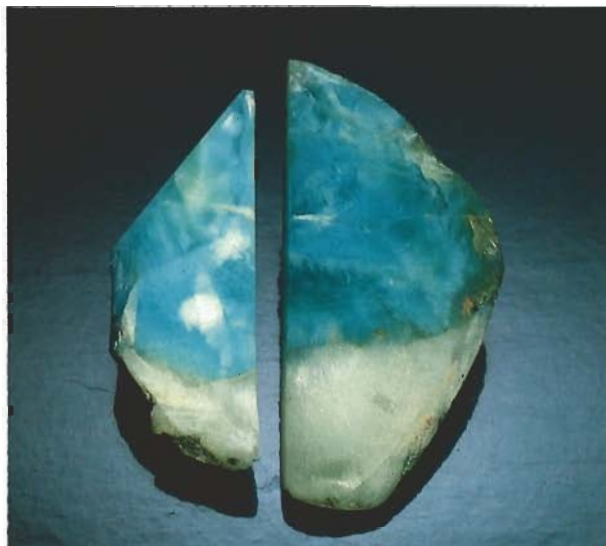
Figure 12. The left part of this pectolite slice was submitted to a jeweler's torch for a few seconds, while the right section remained untouched. The heated section shows a loss of color and transparency that is due in part to the development of small fractures which also reduce the toughness of the specimen. Photo by Robert Weldon.
