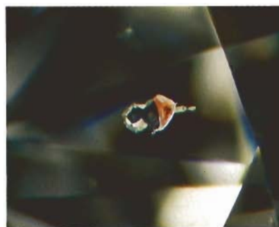
Figure 2. When the host diamond is viewed face up, this included crystal appears to be half black and half orange. Note also the dodecahedral face. Magnified 35\times .
