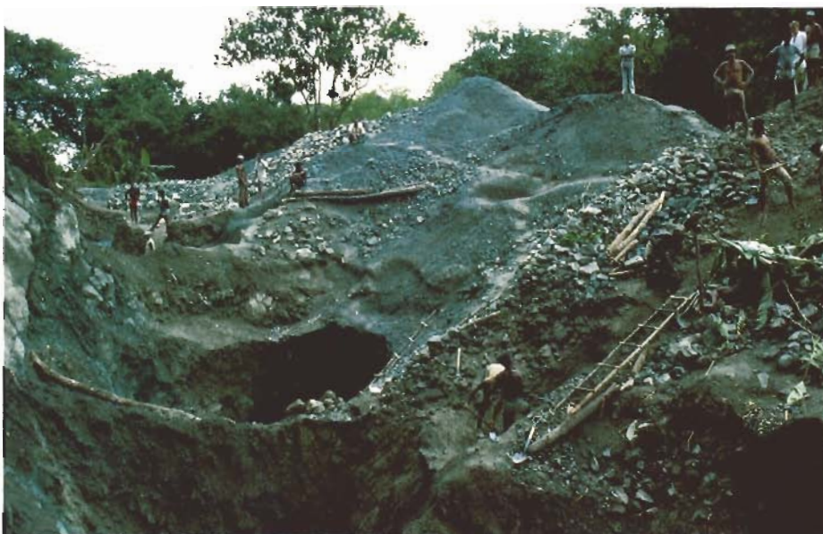
Figure 5. Although much of the area is marked by small pits dug by hand, the newly developed part of the mine uses more sophisticated equipment and techniques to excavate deeper, larger pits in the weathered basalt that hosts the blue pectolite. Photo by Richard Barrett; courtesy of Mountain-Mark Trading Ltd.
