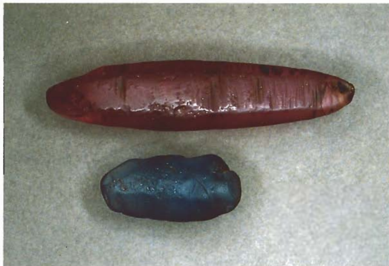
Figure 10. These two apparently waterworn corundum crystals, 56.04 and 21.80 ct, are actually flame-fusion synthetic sapphires. Photo courtesy of the Swiss Foundation for the Research of Gemstones (SSEF).
