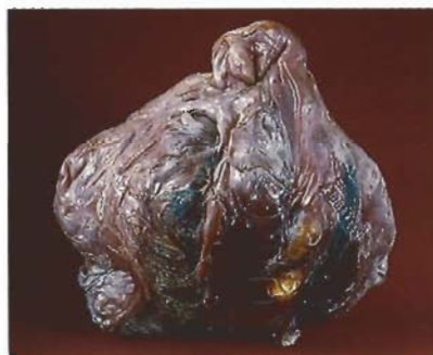
Figure 1. This 28.7 \times 20.5 \times 28.0 cm plastic imitation amber shows numerous gas bubbles and unnatural stamped depressions.
