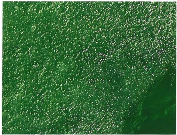
Figure 10. Surface etching was noted on all of the emerald crystals examined. Photomicrograph by John I. Koivula; oblique illumination, magnified 6 \times .
