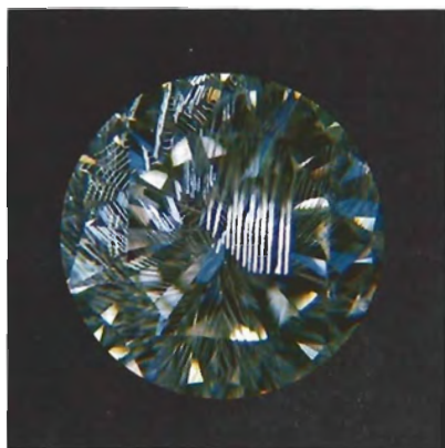
Figure 4. These long, blade-like inclusions produce a kaleidoscopic effect when this 0.75-ct. diamond is viewed faceup. Magnified 16x.
