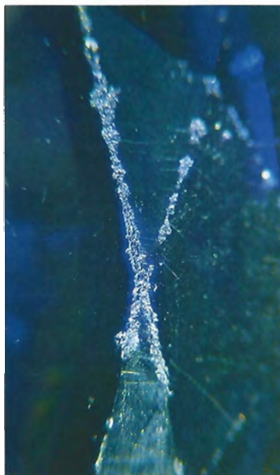
Figure 13. At 35× magnification, the full extent of the abrasion damage to the table facet junctions of the stone shown in figure 12 is apparent.
