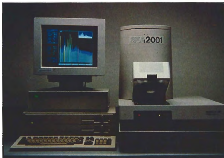
Figure 10. The SEA 2001 Jewelry Assay System for X-ray fluorescence analysis was the most sophisticated method used in this study. The components of this unit are (clockwise from top right): the liquid-nitrogen reservoir that contains the X-ray detector, the sample chamber (on top of the console), a computer, and a monitor (here displaying a typical spectrum). Photo courtesy of Seiko Instruments Corp.
