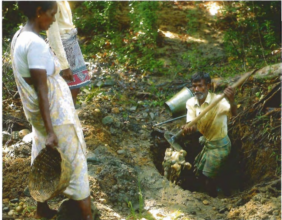
Figure 7. Small-scale mining operations continue in the Elahera gem field of Sri Lanka. This shallow circular pit is located along a tributary of the Mahaweli Ganga River. Photo by Shane F. McClure.
