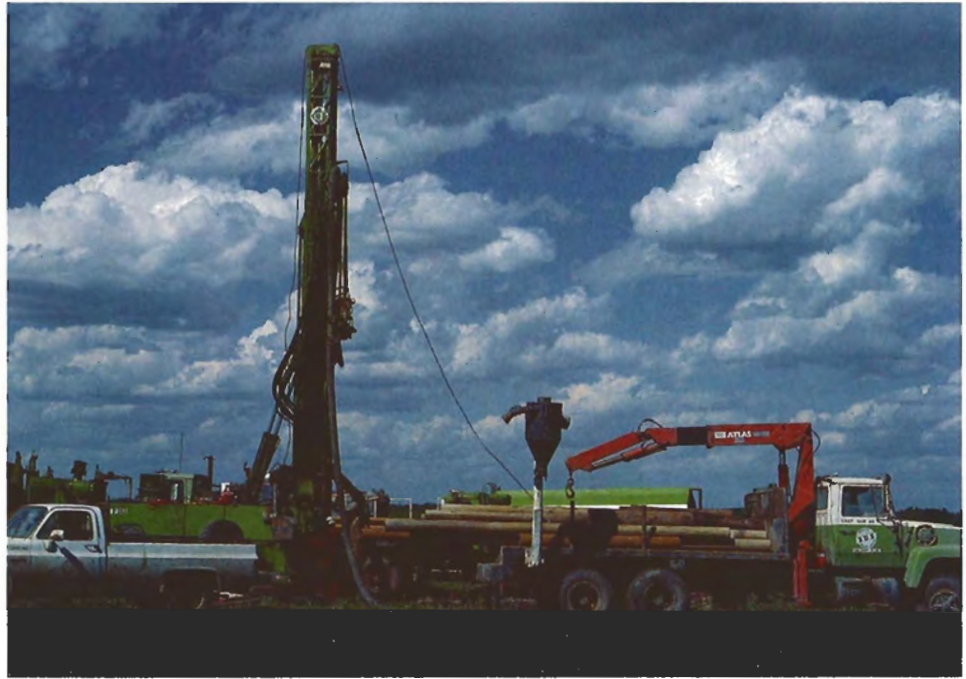
Figure 17. This drilling operation is designed to recover ore from buried kimberlite that has been identified in the Fort à la Corne area of Saskatchewan by geophysical techniques. Note the many meters of drill pipe on the bed of the truck.
