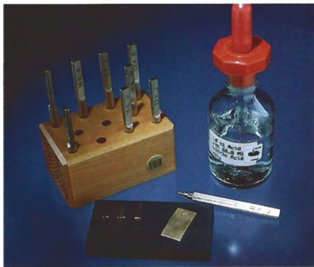
Figure 6. The following tools are needed to determine chemical reactivity by means of touchstone testing on an item believed to be 14k gold (clockwise from upper left): touch needles, 14k acid (43% nitric acid), 14k touch needle, and a basalt touchstone. Note the streaks with acid next to the test piece on the touchstone. Photo by Maha Smith-DeMaggio.
