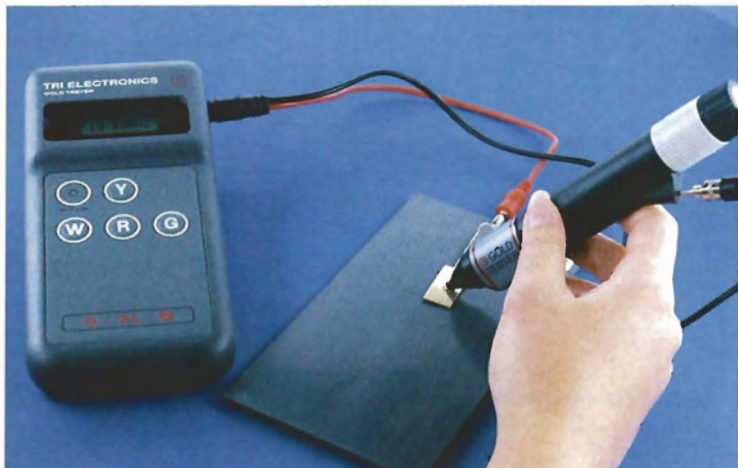
Figure 8. The components of the G-XL-18 Gold Tester, used for capacitive decay testing, include (from left to right): the G-XL-18 tester unit, an electrical hook-up with test piece and electrolyte gel, and a gel dispenser/probe wand. For this test, the operator positions the test piece in the clip and applies a drop of gel. With the probe touching the gel, the operator then presses the button that corresponds to the color of the test piece. The results are displayed on the tester unit. Photo by Maha Smith-DeMaggio.
