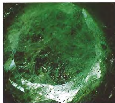
Figure 6. Note the large gas bubble in the filling material that was used to clarity enhance this 8.02-ct emerald. Magnified 9 \times .
