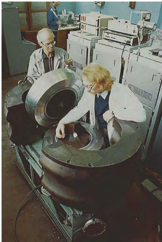
Figure 2. A "split sphere" apparatus is used to grow synthetic diamond crystals at Novosibirsk. Left: This view of the apparatus opened reveals the internal spherical cavity, which holds the two sets of anvils and the central high-pressure cell. Right: The same apparatus is in a closed configuration at the start of an experiment to grow diamond crystals. Photos provided by N. V. Sobolev.
