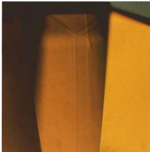
Figure 11. A different kind of internal graining, also in the form of intersecting lines, is seen through the pavilion facets of the same synthetic diamond shown in figure 10. Photomicrograph by John I. Koivula; magnified 40 \times .
