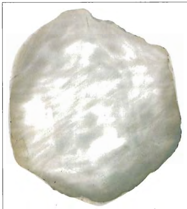
Figure 10. Overreduction of high-iron sapphire, such as that from Rock Creek, leads to hercynite precipitation; this makes the material, like the sample shown, a translucent gray. Prior to heat treatment, this wafer (5 mm in diameter and 0.34 mm thick) was colorless and transparent. Photo © John L. Emmett.
