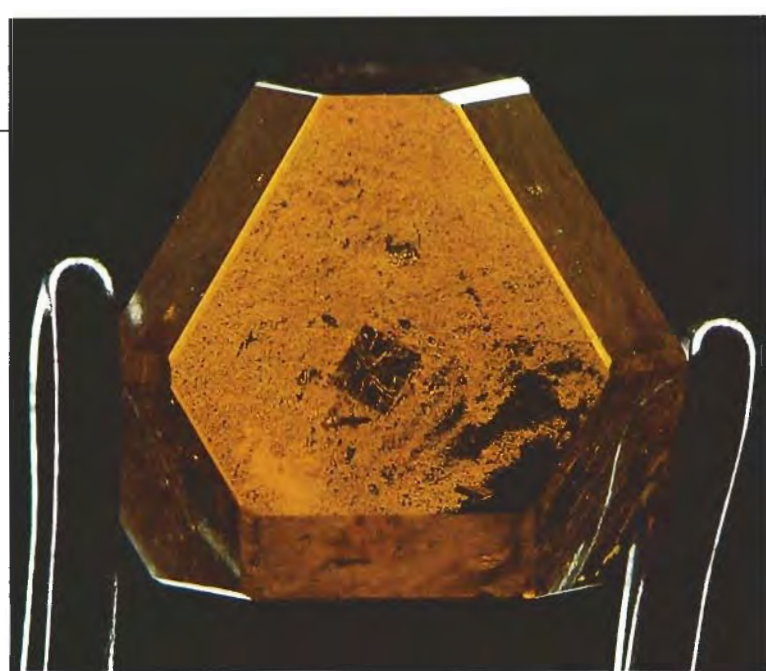
Figure 4. This 0.78-ct synthetic diamond crystal (no. 21476) shows the arrangement of crystal faces and the location of the seed (the black-appearing square area) on the octahedral face at the base of the crystal. Photomicrograph by John I. Koivula.
