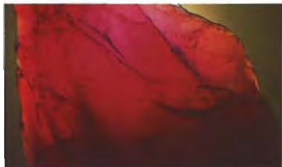
Figure 12. The curved striae in this 18.45-ct synthetic ruby, which was misrepresented as natural Vietnamese rough, became readily apparent when the stone was examined using combined brightfield illumination and immersion. Magnified 10x.
