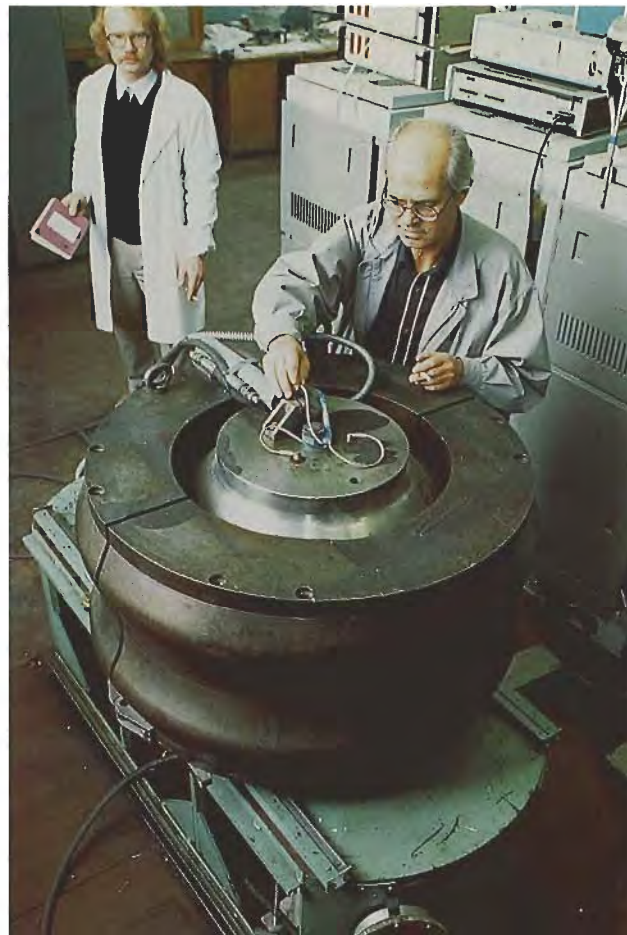
Figure 2. A "split sphere" apparatus is used to grow synthetic diamond crystals at Novosibirsk. Left: This view of the apparatus opened reveals the internal spherical cavity, which holds the two sets of anvils and the central high-pressure cell. Right: The same apparatus is in a closed configuration at the start of an experiment to grow diamond crystals. Photos provided by N. V. Sobolev.
