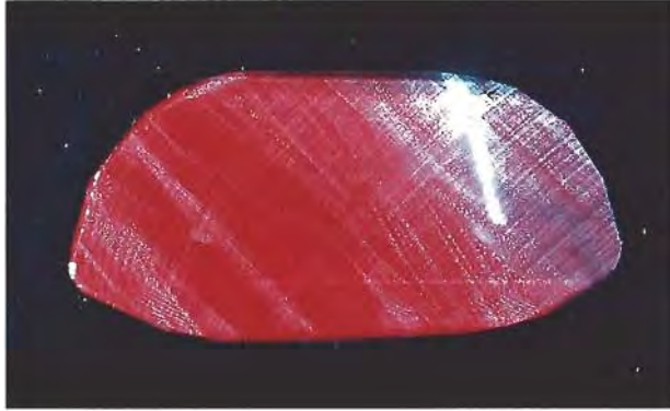
Figure 17. This laser-tomographic image of a 0.68-ct synthetic ruby shows the growth banding characteristic of flame-fusion synthetics as well as the treatment-induced "fingerprints" that result from flux overgrowth. Photo courtesy of Junko Shida.
