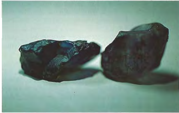
Figure 7. These two synthetic sapphires (19.20 and 29.90 ct) were sold as natural sapphire rough in Vietnam. Photo by Tony Laughter.
