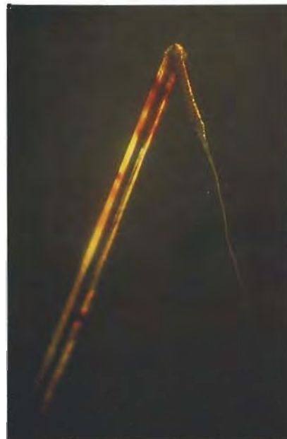
Figure 4. A series of brown radiation stains were noted along the length of this etch tube in a 2.37-ct fancy dark yellowish brown diamond. Magnified 35 \times .
