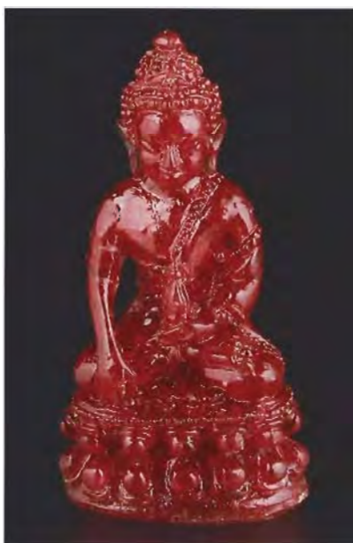
Figure 1. Testing revealed that this Buddha statuette (about 41.60 × 21.40 × 16.20 mm) is an assemblage of ruby and pink corundum chips in plastic.
