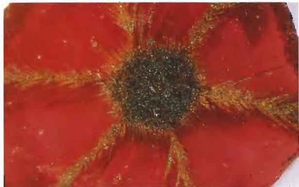
Figure 10. In reflected light, this trapiche ruby slab reveals a series of parallel tube-like structures extending outward from each of the six arms of the star and from the dividing planes between the black core and the six trapezoidal red zones. Magnified 10×.
