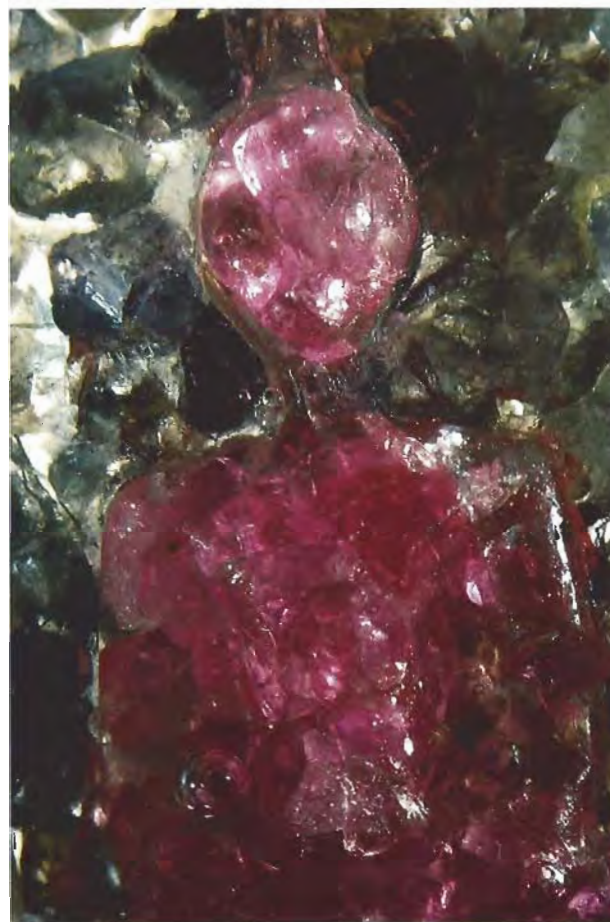
Figure 10. With magnification, gas bubbles can be seen in the polymer matrix. The grains in the pink region appear to be synthetic ruby and synthetic pink sapphire; in the green region, some of the corundum grains show evidence of heat treatment. Photomicrograph by John I. Koivula, magnified 5 \times .
