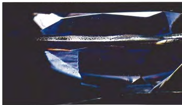
Figure 16. In profile, the bottom of the "glue" layer of the pear-shaped triplet in figure 15 can be seen as a faint line near the top of the pavilion. Photo by Maha DeMaggio.
