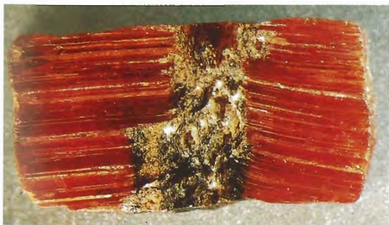
Figure 14. In this view of a 5.9-mm-diameter trapiche ruby crystal parallel to the c-axis, the tube-like inclusions show a small inclination to the basal plane.
