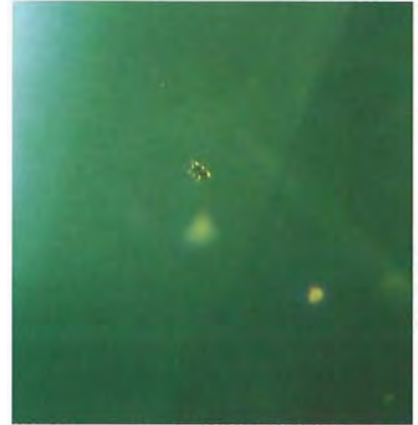
Figure 8. At lower magnification, this gold-colored plate-like inclusion in the synthetic emerald in figure 7 resembled pyrite, a mineral found in some Colombian emeralds. Magnified 200 \times .
