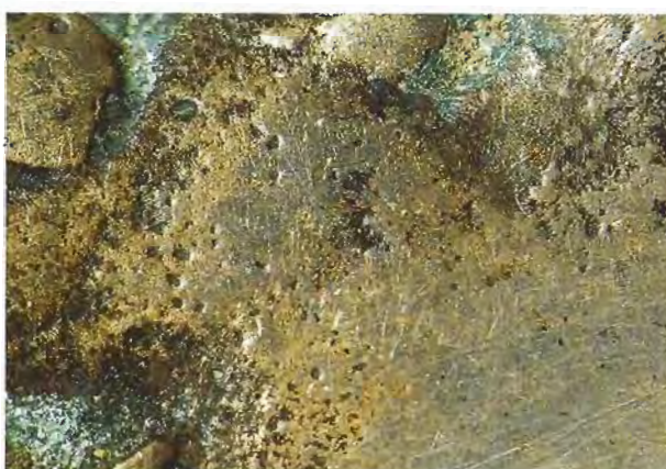
Figure 13. With magnification, the metallic brooch in figure 12 appeared brown, with a greenish patina in some regions. Chemical analysis confirmed that the material was not a nickel-iron meteorite but rather a copper alloy. Photomicrograph by John I. Koivula; magnified 10×.
